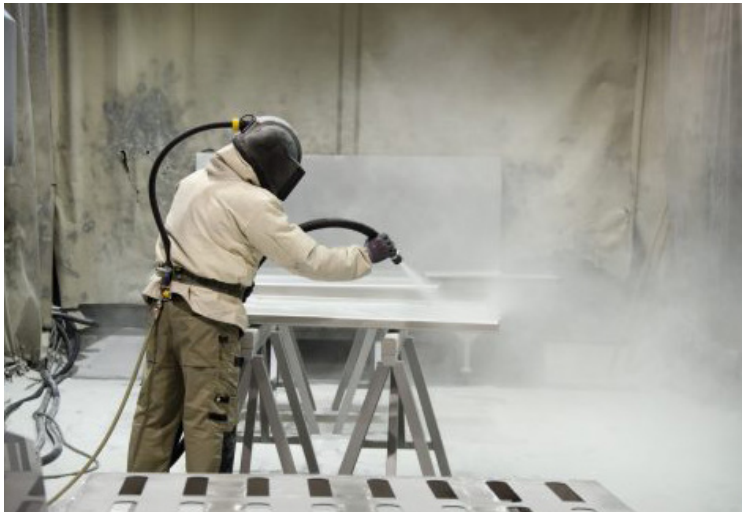
sandblasting steel structures © coating.nl
