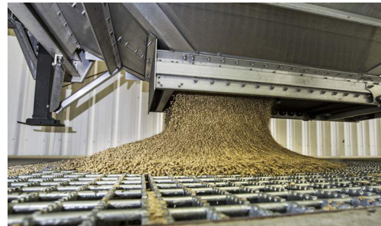
MDF board production - adding resin © Action Tesa
