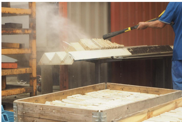
cleaning of reclaimed ceramic tiles © RotorDC
