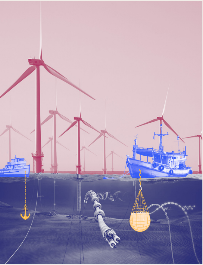
Figure 3: Fishing vessels damaging wind farm cables with their anchors and nets Source: Freepik, techxplore.com
