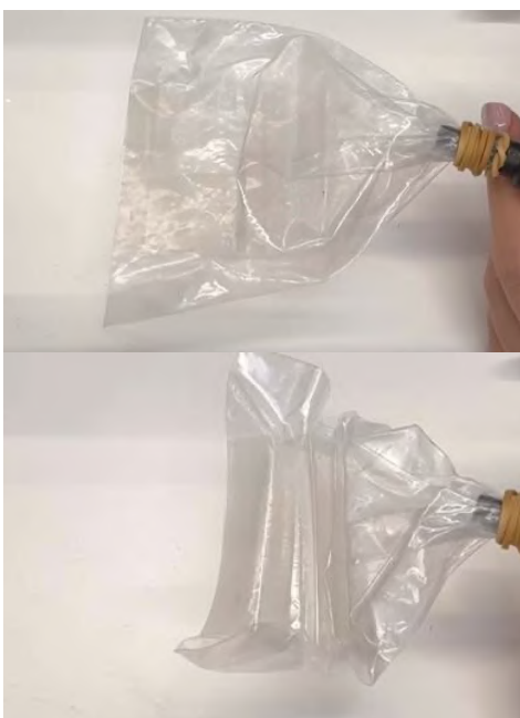
Figure 27. Vacuum-driven origami test
