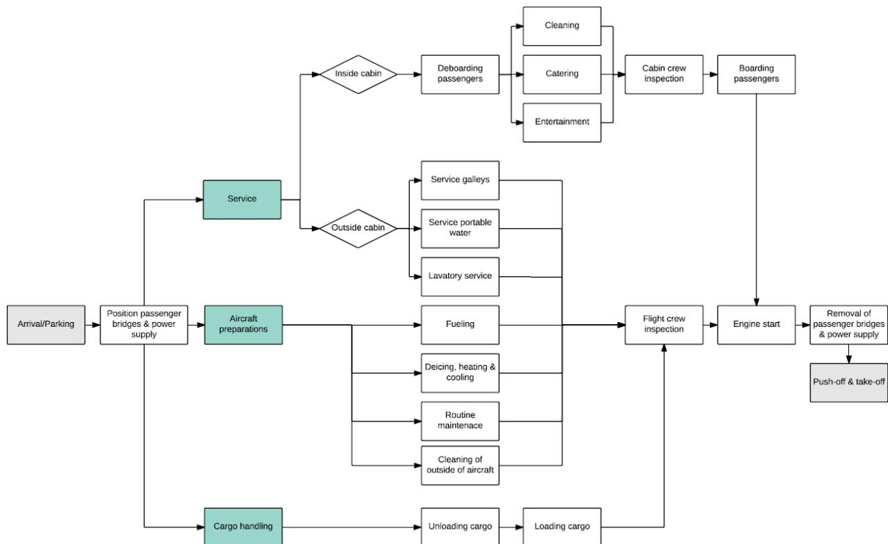
Figure 13.1: Work flow diagram for ground operations [101]
