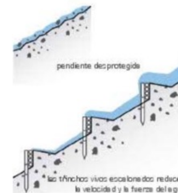
Slope stabilization by local material & simple construction technique
