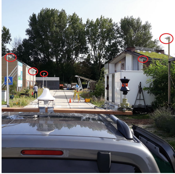
Fig. 3.2 Set-up of the prototype SuperGPS system at The Green Village on the TU Delft campus
