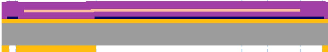
4. Ceramic stack patterning and bond pad/electrode opening
