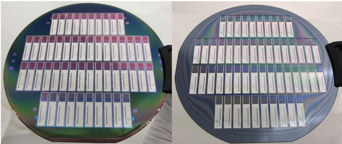
*Figure 30: Devices still in silicon frame from (a) the front side of the wafer; (b) the back side of the wafer.*
