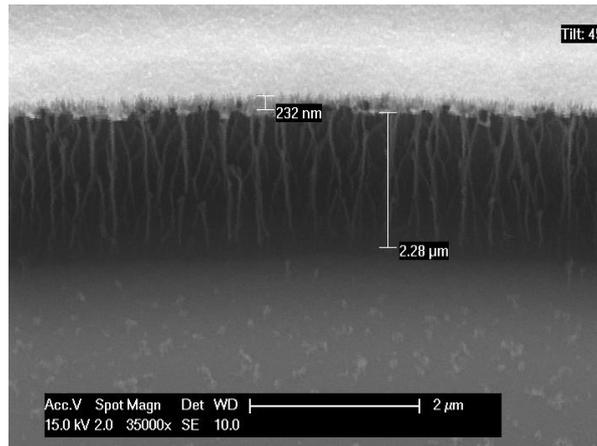
Figure 14: SEM photo of wet etched structure sidewalls with visible residues on  $\text{SiO}_2$ .
