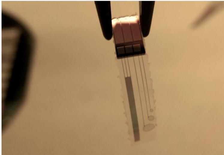
Figure 32: Released device cut out from the silicon frame.
