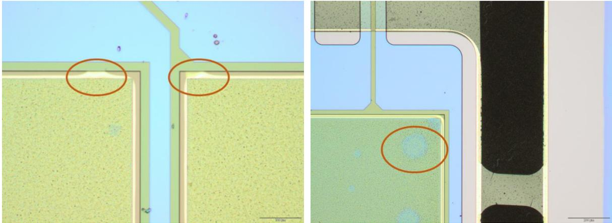
*Figure 23: (a) Visible etching or delamination of TiN layer beneath the parylene encapsulating layer indicated; (b) Visible uneven spots on the TiN bond pad indicated.*
