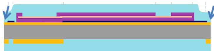
Figure 61: Arrows indicate where parylene layer thickness may be measured using LEITZ.
