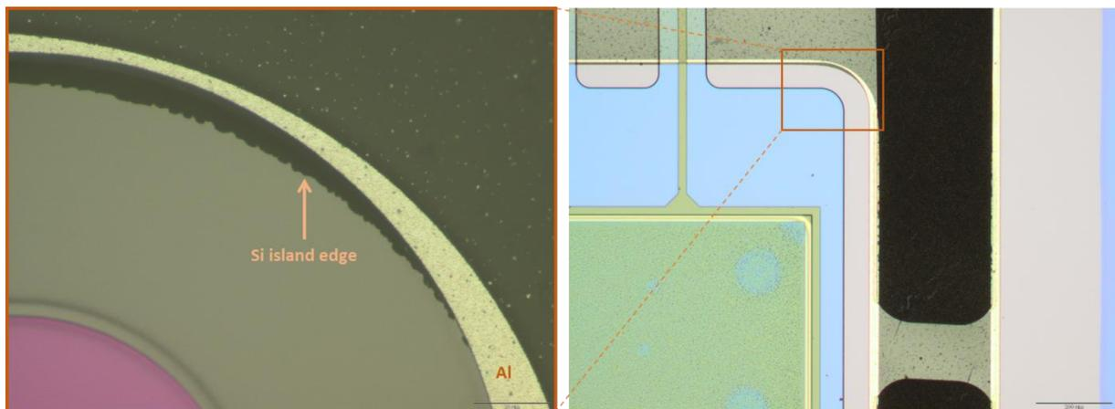
Figure 28: (a) Gap between DRIE silicon island and remaining Al etch stop; (b) Gap between DRIE silicon and Al etch stop zoomed out.
