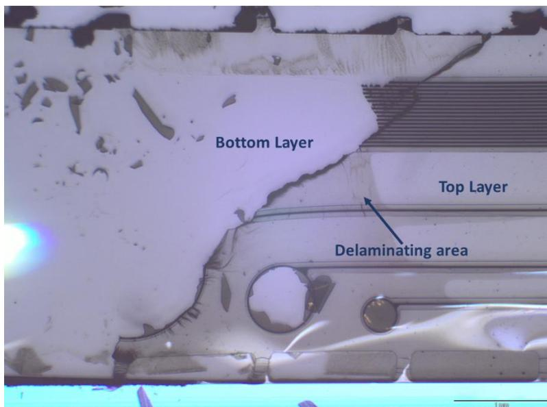
Figure 38: Section of device with torn off top parylene layer.
