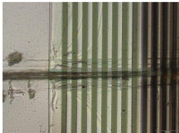
*Figure 53: Test device that was folded and flattened completely.*
