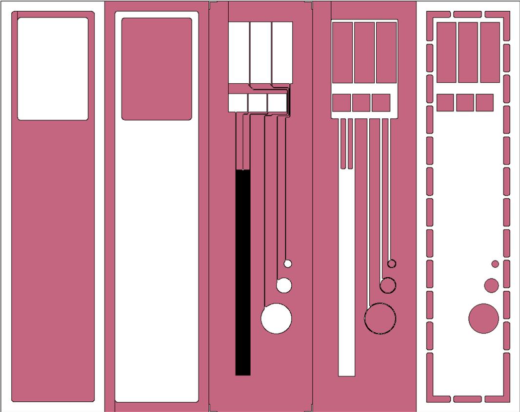
Figure 6: Masks for (a) hard mask for DRIE; (b) Al etch stop layer; (c) metallization; (d) ceramic layers; (e) Ti buried mask.
