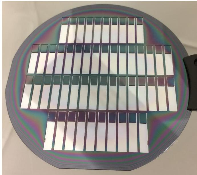
*Figure A.56: DRIE done on a wafer with the rounded release mask with no broken membranes.*
