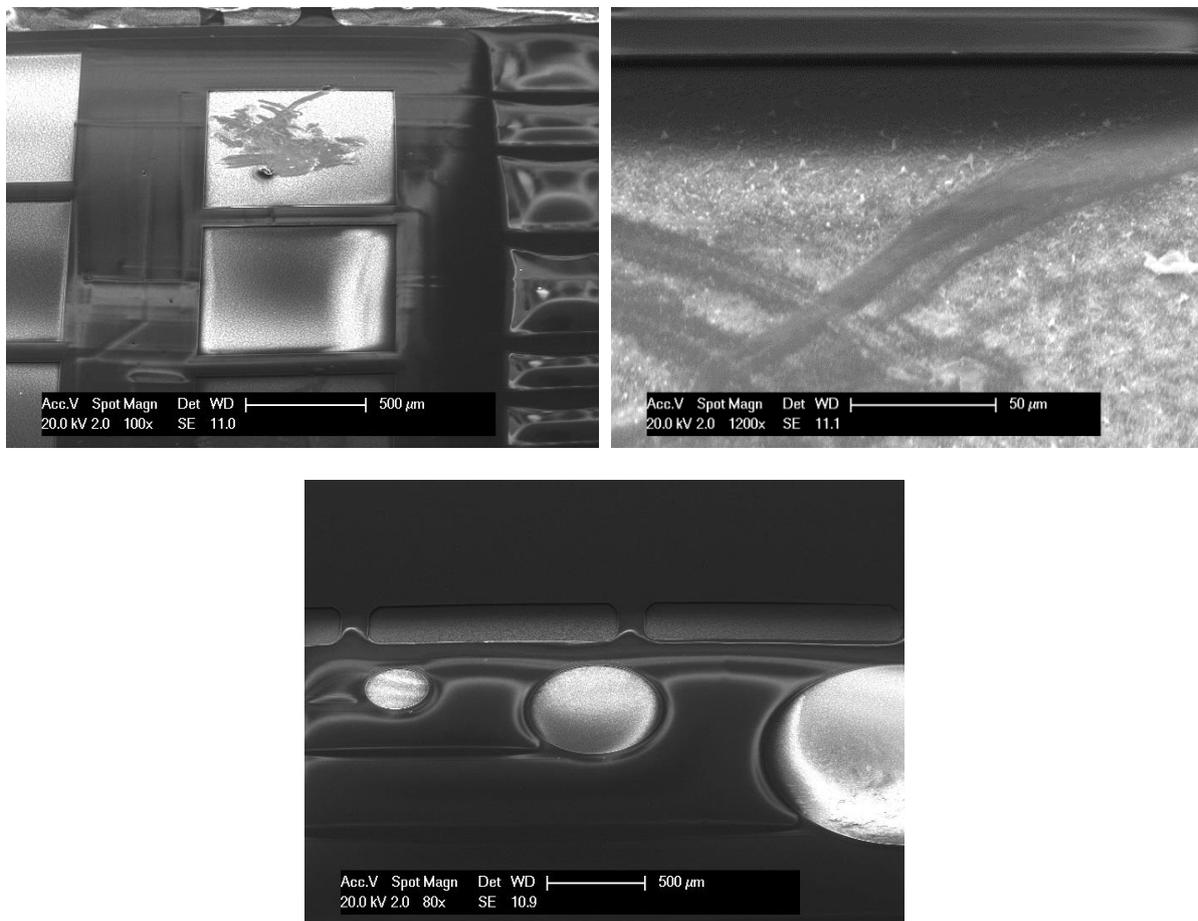
*Figure 35: (a) SEM photo of a charging layer of residue on bond pads on a Si island with scratches made by probe needle; (b) Close up of the surface of a bond pad from (a); (c) SEM photo of charging layer of residue on the bond pad on a flexible membrane.*
