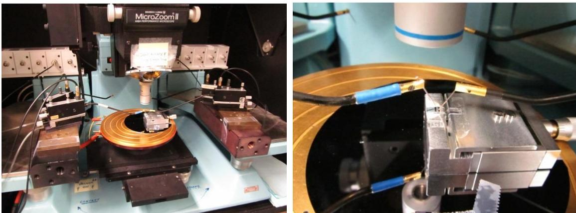
*Figure 48: Bending tool on carrier wafer on the probe chuck with needles touching down on the bond pads.*
