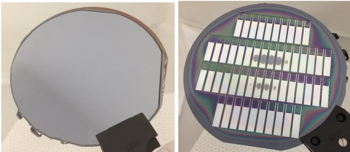
Figure A.58: Wafer misalignment after etch due to heating of wax from (a) the front side; (b) the back side. The center of the wafer shows some unetched oxide, but the DRIE was not completed.
