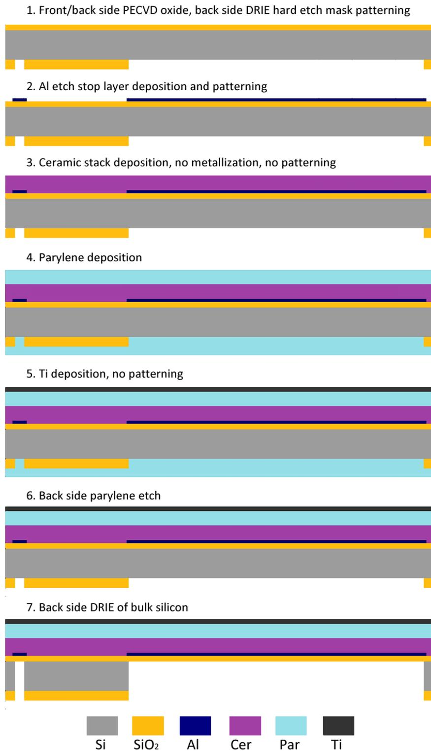
Figure A.55: Process flow for preparing DRIE test wafers.
