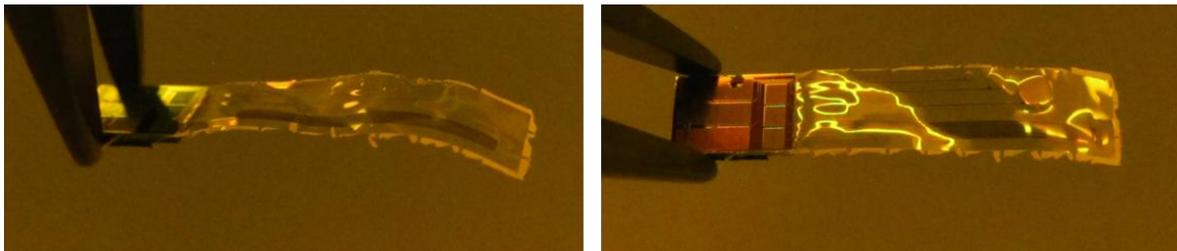
Figure 45: Device 5 from Batch 2 showing wrinkling in the parylene membrane after being soaked for 4 weeks.
