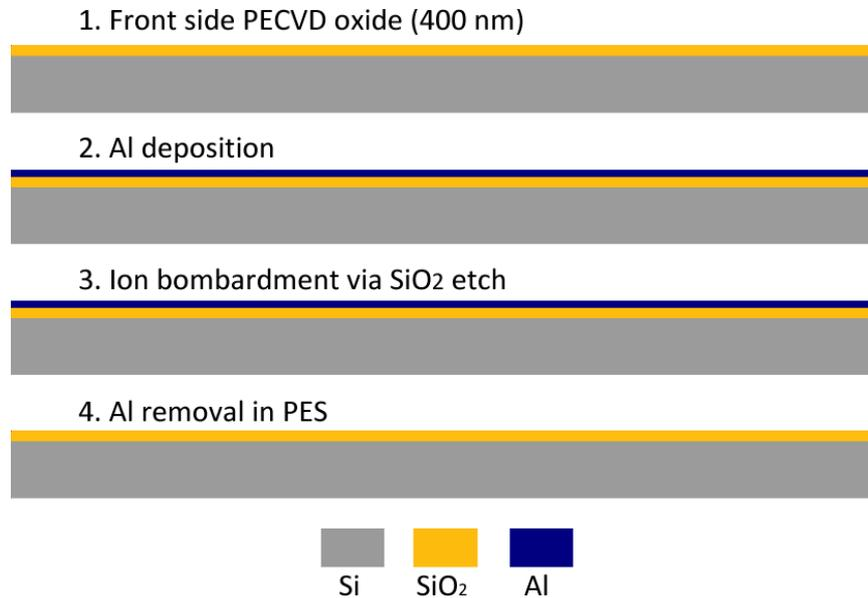
Figure 17: Aluminum etch stop layer short loop schematic.
