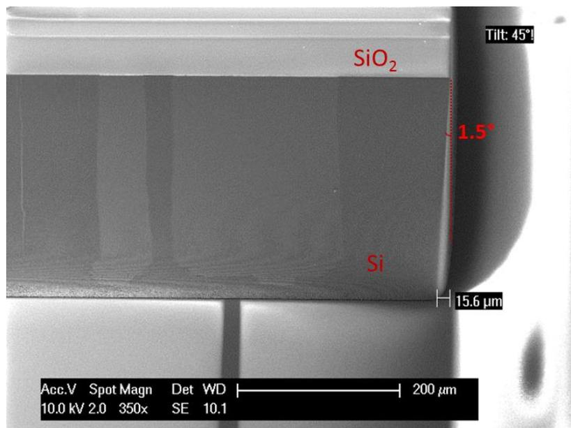
Figure 27: SEM photo showing negative sloping when bulk silicon is etched.
