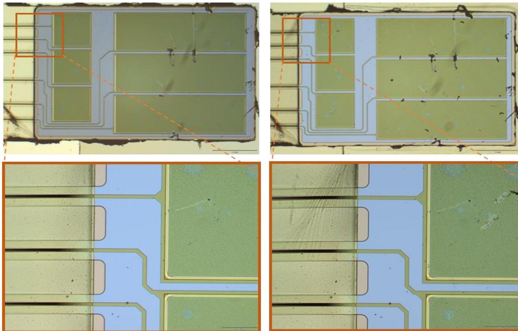
Figure 43: Device 1 at (a) 0 hours; (b) 6 hours with visible cracks in the membrane at the edge of the silicon island due to handling.
