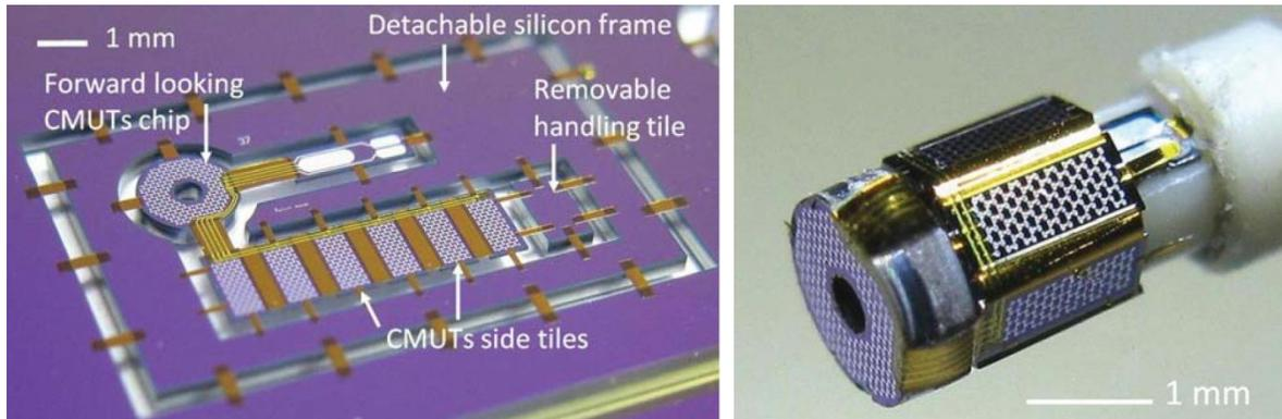
Figure 2: (a) F2R demonstrator in silicon frame; (b) Demonstrator released from the frame and integrated at the tip of a catheter [10].
