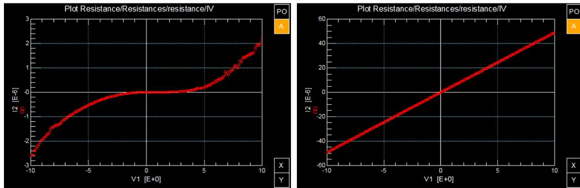
Figure 44:  $I$  vs.  $V$  curves at 4 weeks for (a) Device 1 showing nonlinear resistance over the voltage sweep; (b) Device 2 showing linear resistance over the voltage sweep.
