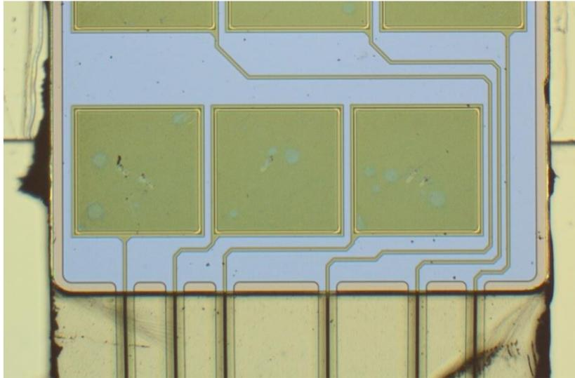
*Figure 25: Location of where cracks spread from the corners of the silicon island where the edge meets the parylene membrane. Note that this image is of a device made with the rounded back side DRIE hard etch mask and not the prototype device.*
