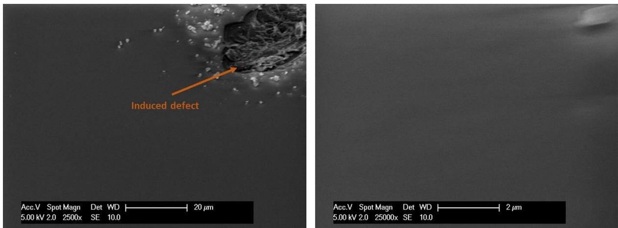
Figure 21: Wafer 4 (200 nm at 300°C) – induced defect and charged particles, no defects.
