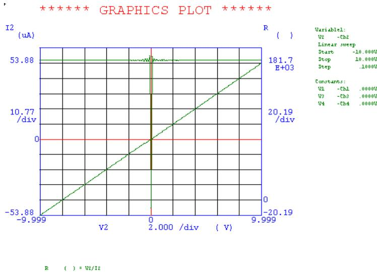
Figure 49: I vs. V plot for Device 1 with a bending radius of 2mm (beginning of test).
