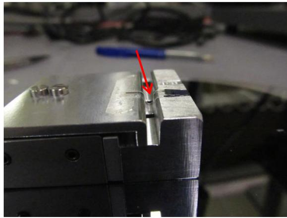
*Figure 47: Bending tool with a device affixed and the membrane placed in a gap of 2 mm*
