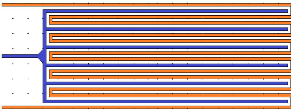
Figure 4: An example of comb (blue) and meander (orange) structures.
