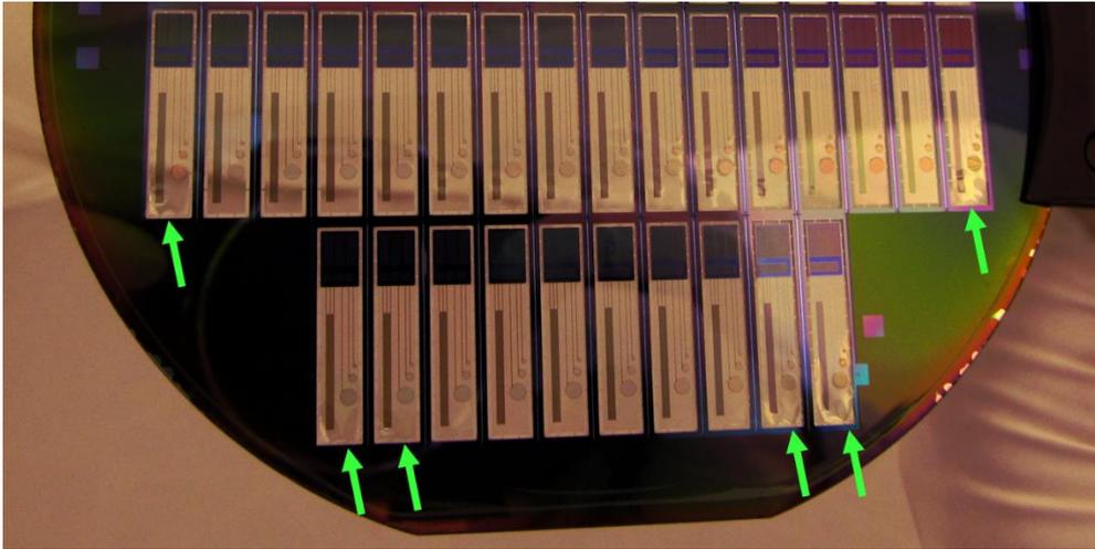
Figure 36: Dies with delaminating parylene membranes indicated with arrows.
