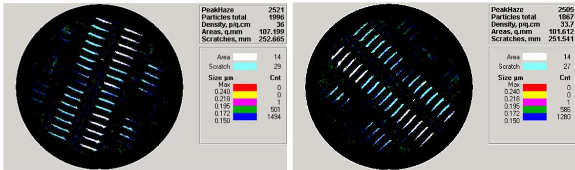
Figure 9: Scratch and particle count (a) before etch; (b) after etch.
