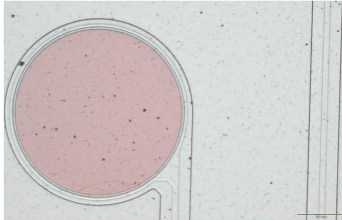
*Figure 33: Front side of device showing TiN on electrode bond pads.*
