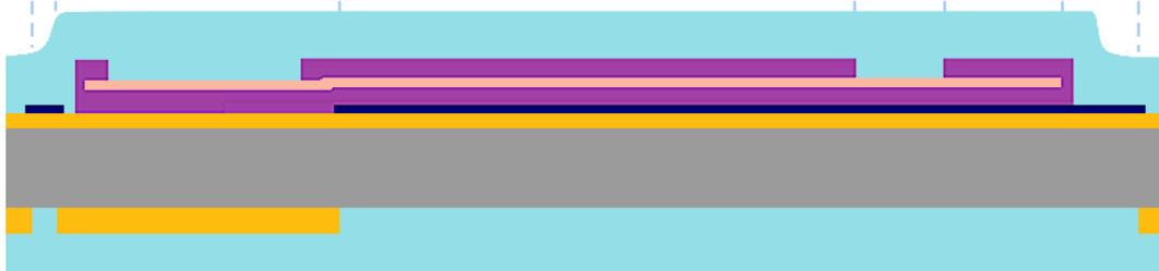
6. Ti buried mask dep, back side parylene etch, Ti patterning
