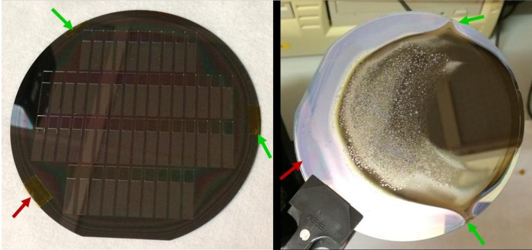
Figure A.59: (a) Process wafer with back side up taped where indicated to carrier wafer; (b) Front side of wafer after DRIE with removed Ti.
