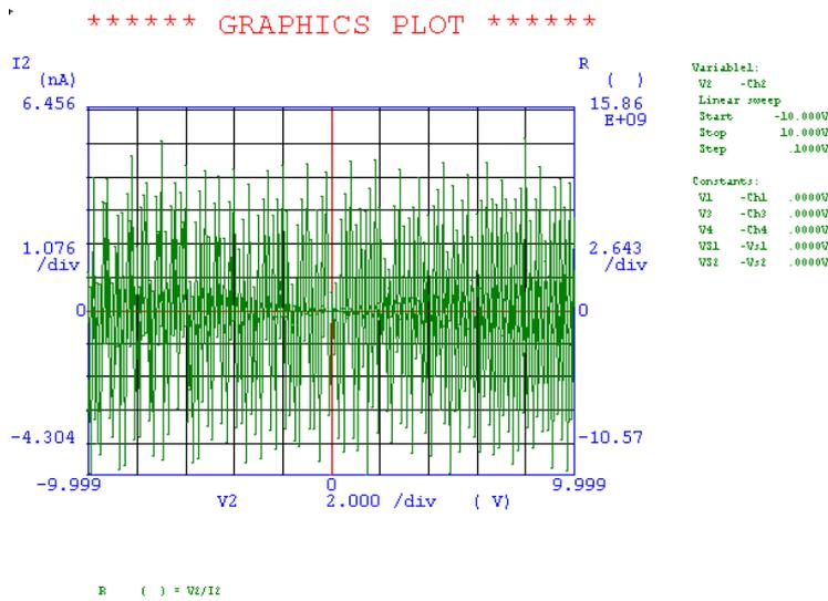
Figure 50: I vs. V plot for Device 1 with a bending radius of 0.15mm (on failure).
