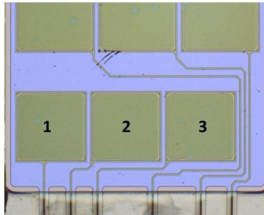
Figure 41: Labelled bond pads of the meander (1 and 3) and the comb (2).
