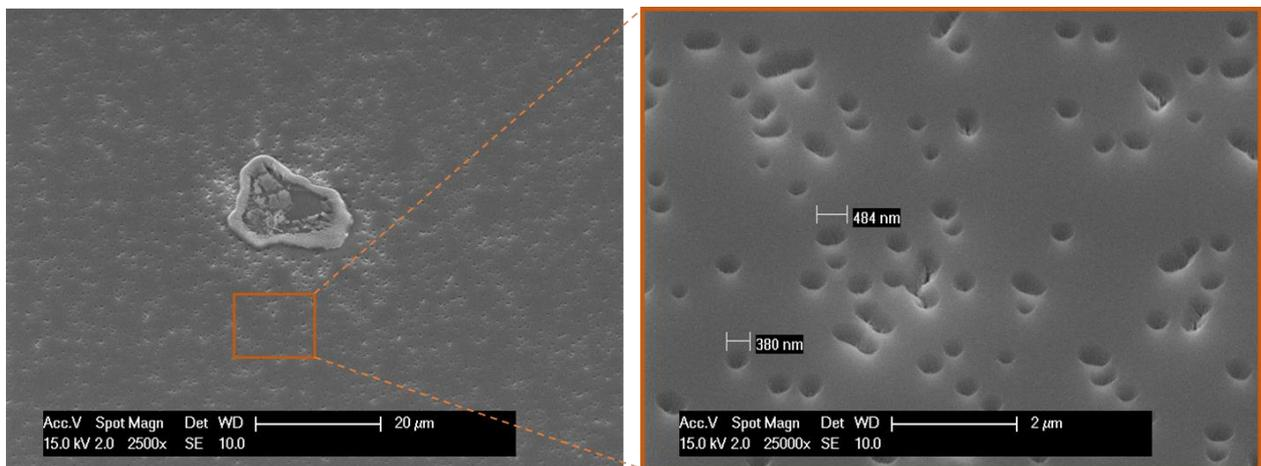
Figure 19: Wafer 2 (100 nm at 350°C) – frequent defects of ~400nm.
