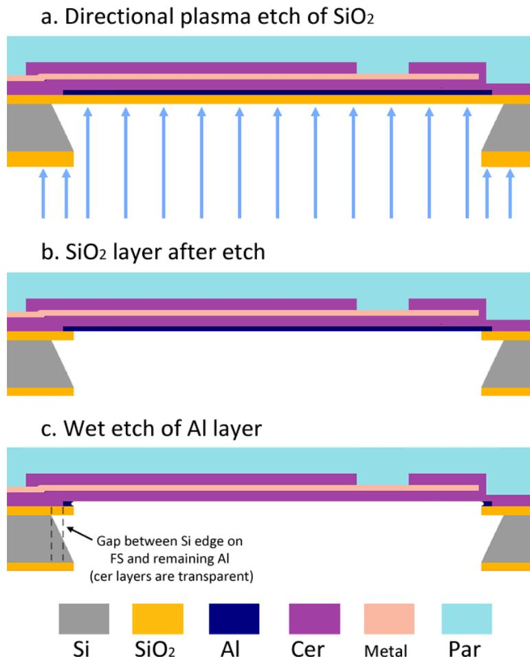
Figure 29: (a) Direction of dry etch to remove  $\text{SiO}_2$  layer after DRIE (Step 7 in the full flowchart); (b) Al etch stop layer exposed after  $\text{SiO}_2$  is etched; (c) the device after Al wet etch, with the location of the gap between Si edge and visible Al indicated. Angle of Si sidewalls is exaggerated.
