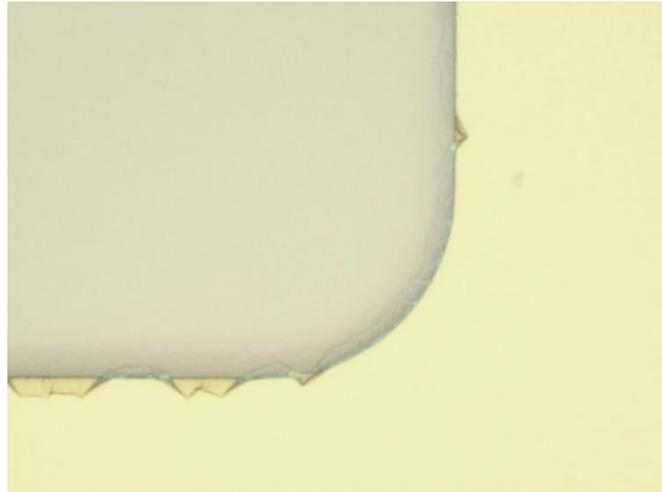
*Figure 10: Photoresist residue film clinging to edges of structures.*
