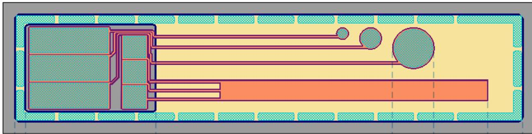
1. Front/back side PECVD oxide, back side DRIE hard etch mask patterning
