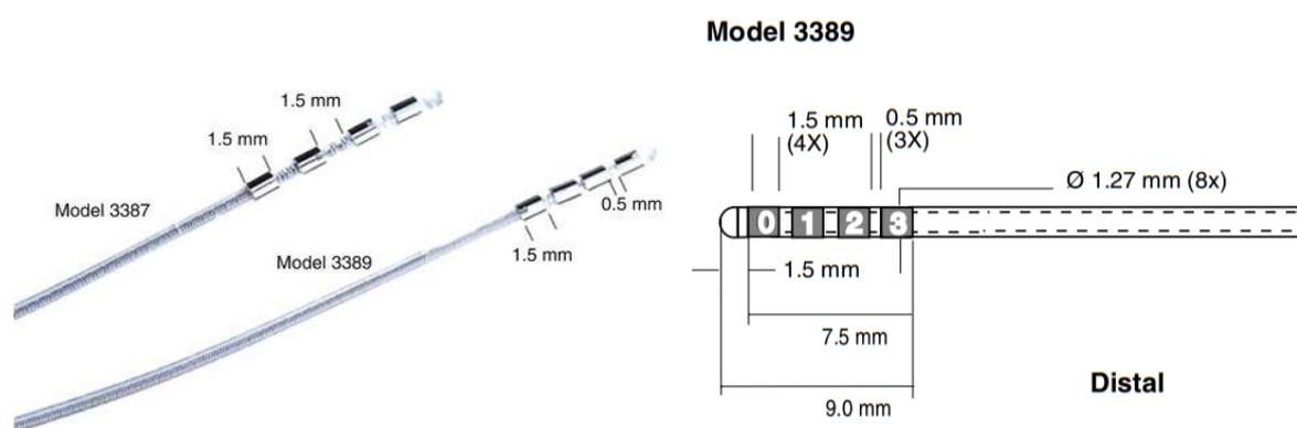
Figure 1: Electrodes on Medtronic lead model 3389 for DBS [4],[5].
