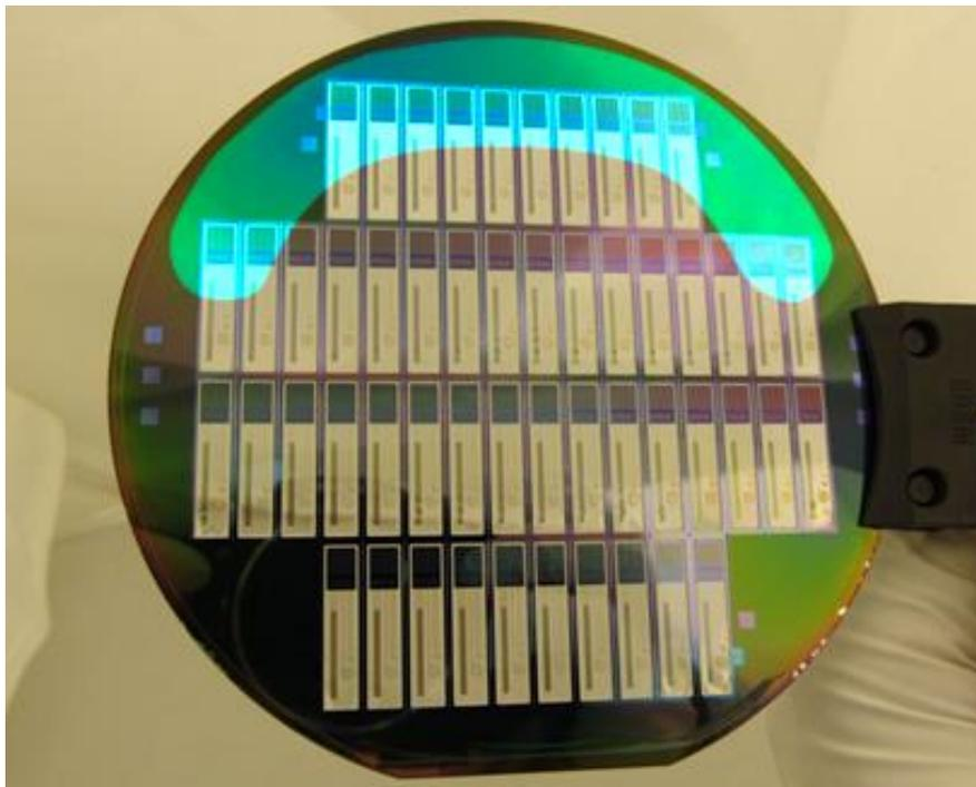
Figure 42: Highlighted area of the wafer that showed the most dies with high meander resistances ( $\sim 300 k\Omega$ ).
