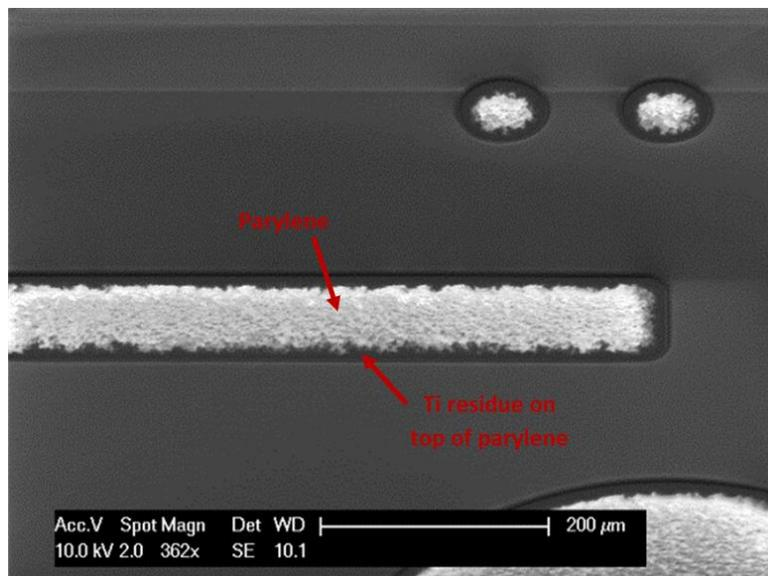
Figure 15: SEM photo of Ti residue around the edges of structures.
