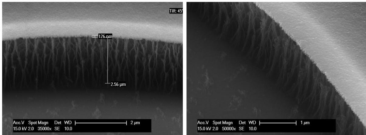
Figure 16: SEM photo of (a) dry etched structure sidewalls and (b) Ti mask edge.
