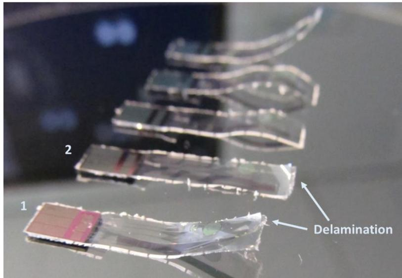
Figure 46: Delamination of parylene layers on Device 1 and 2 of the reference batch.
