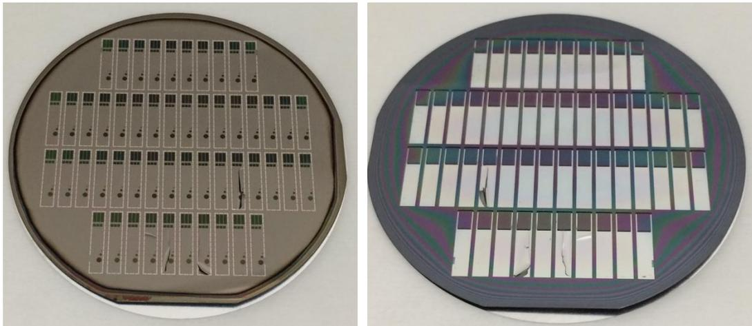
*Figure A.54: Front side and back side of a wafer after DRIE with broken membranes. The back side DRIE hard mask used was the first version, with no rounded corners.*
