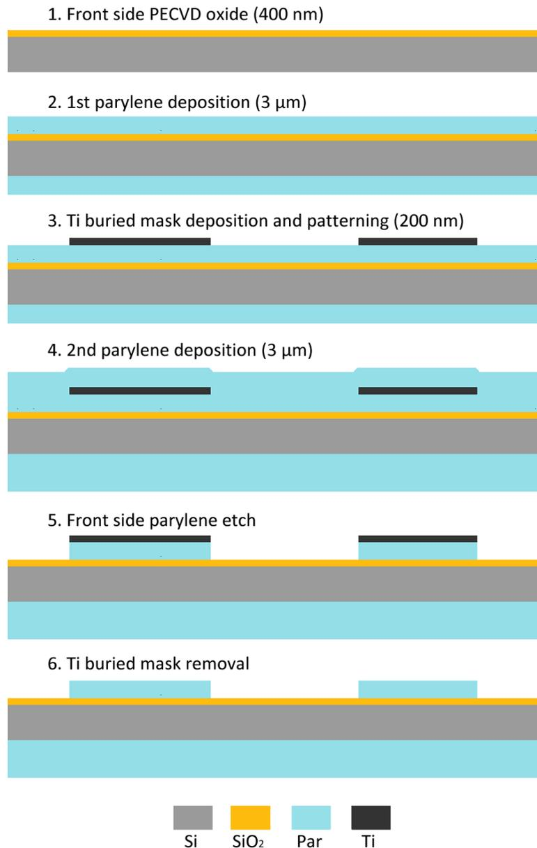
Figure 8: Ti buried mask short loop schematic.
