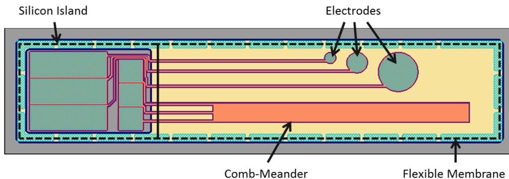
Figure 3: Labelled structures of the device.
