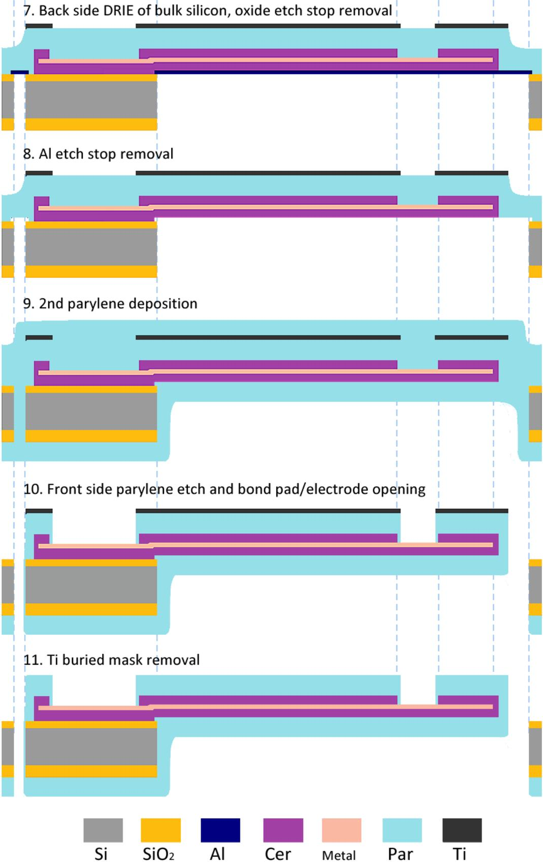
Figure 5: Simplified schematic flow of the full process.
