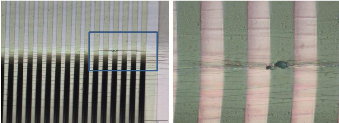
*Figure 52: Device 2 after having been bent to .2 mm.*
