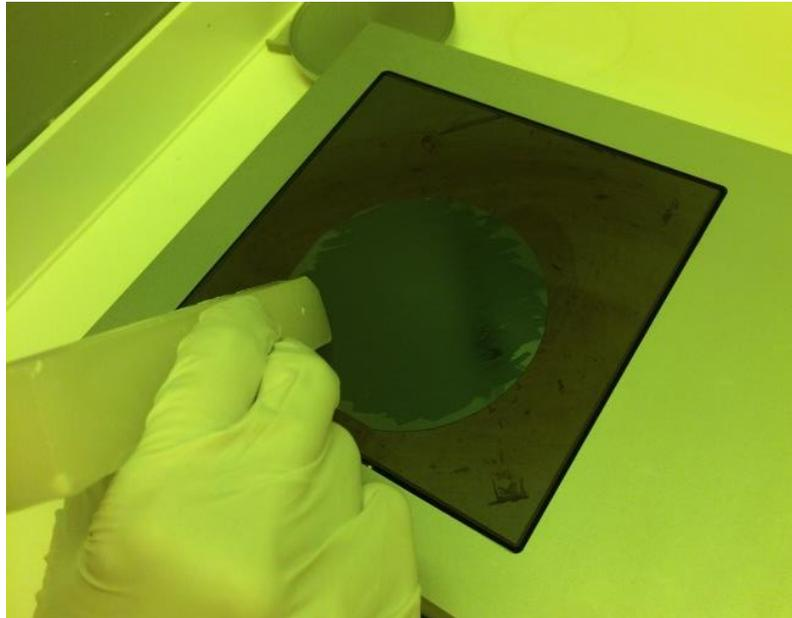
Figure A.57: Applying wax to carrier wafer.
