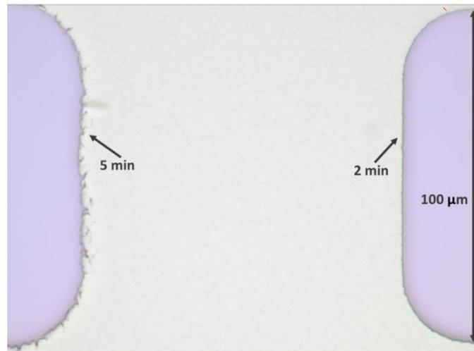
Figure 12: Structure edges after 5 minutes and 2 minutes in SC-1 etchant.
