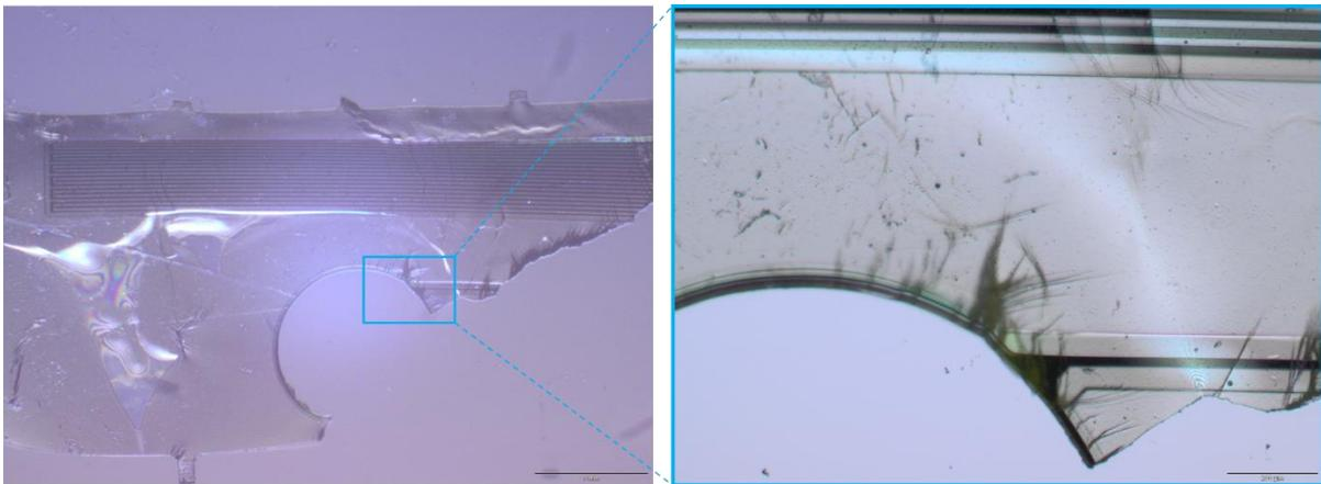
Figure 37: Top layer of parylene with metallization and ceramic encapsulation.
