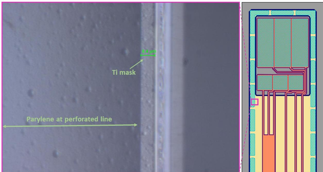
Figure 26: Ti buried mask for parylene etch overlapping the released area.
