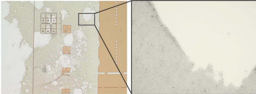
*Figure 11: Film of Ti residue seen after HF etch on top of parylene around structures.*
