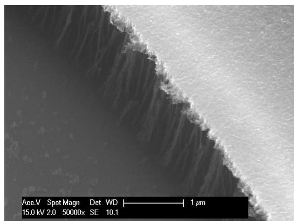
Figure 13: SEM photo of wet etched Ti edge.
