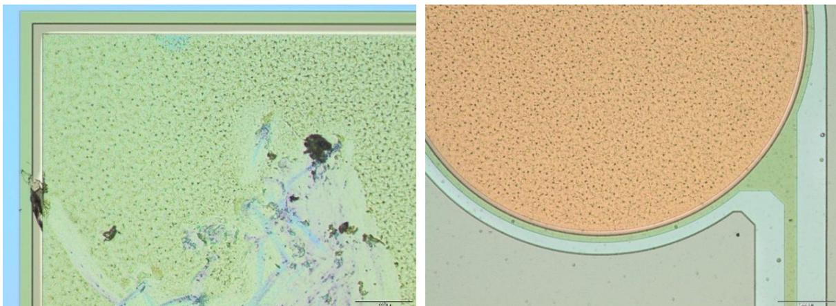
*Figure 34: (a) Layer of residue on bond pad on Si island with scratches made by probe needle; (b) Layer of residue on bond pad on flexible membrane.*
