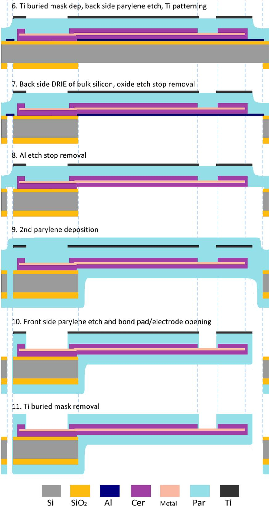
Figure 24: Simplified schematic flow of the full process.
