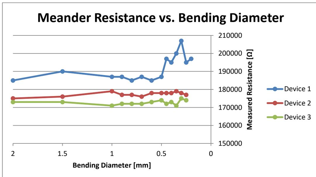
Figure 51: Resistance vs. bending diameter.
