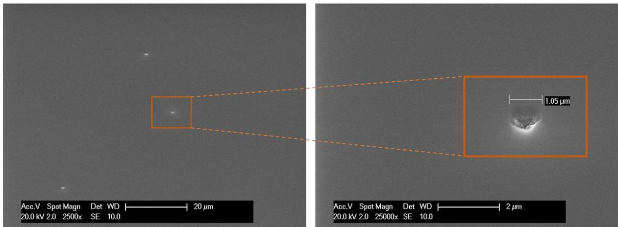
Figure 18: Wafer 1 (60 nm at 25°C) – rare defects of ~1µm.
