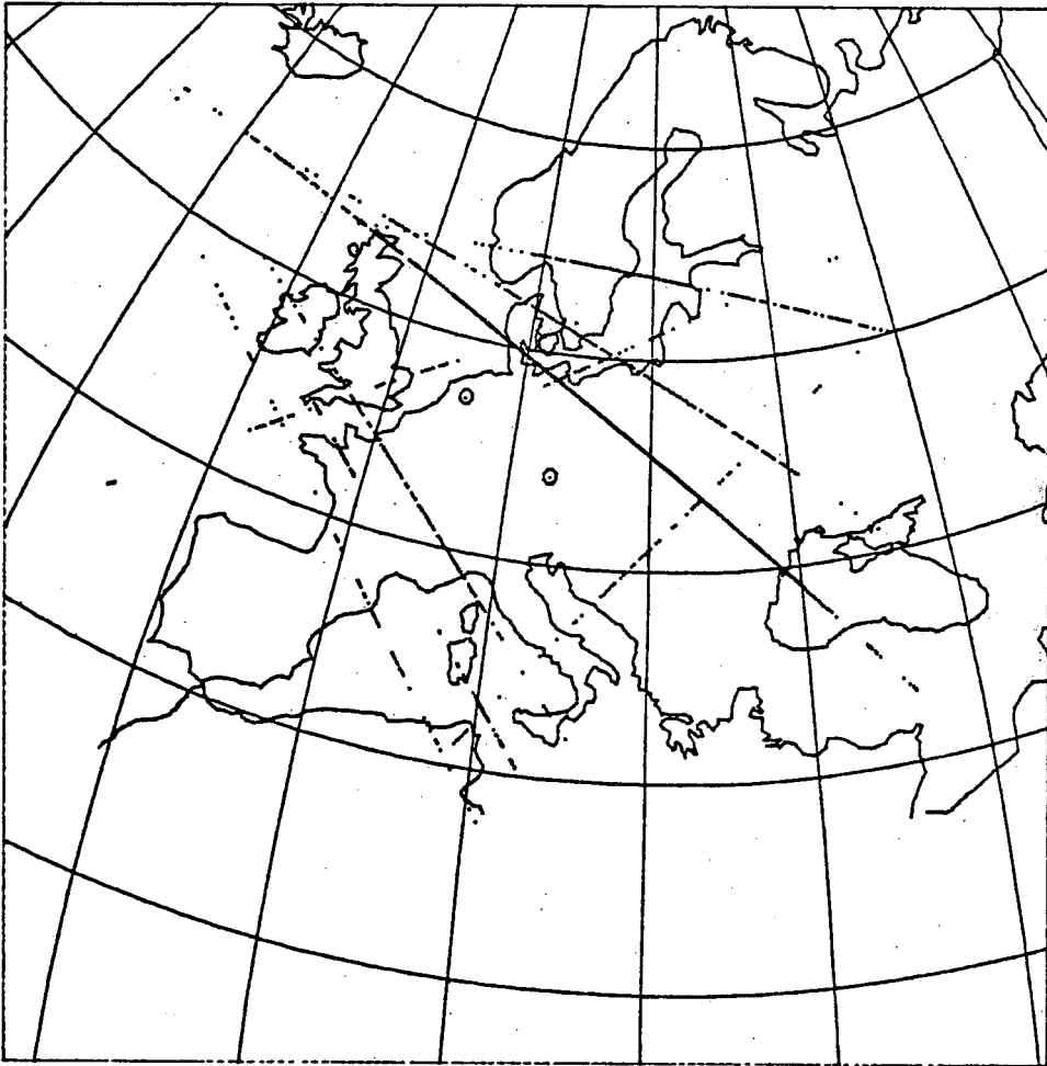
Fig. 5: The sub-satellite points at the observation times for all passes in arc 4 (GEOS 1). The general direction of the satellite motion is from west to east.
