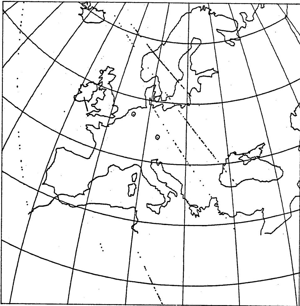
Fig. 3: The sub-satellite points at the observation times for all passes in arc 2 (LAGEOS). The satellite moves from south to north.
