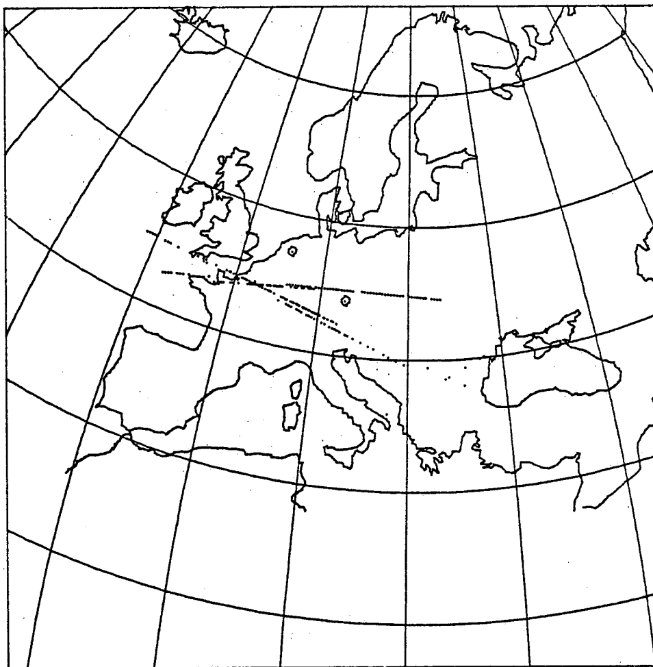
Fig. 4: The sub-satellite points at the observation times for all passes in arc 3 (STARLETTE). The satellite moves from west to east.
