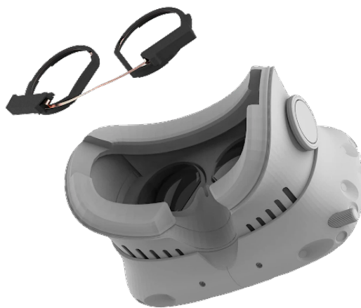
Figure 3.2: Pupil Labs binocular eye tracking add-on for VIVE Pro
