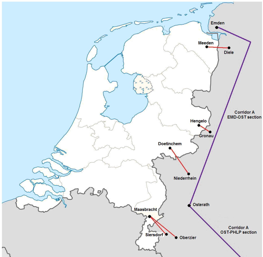
Fig.4.26 Interconnection buses between the Netherlands and Germany
