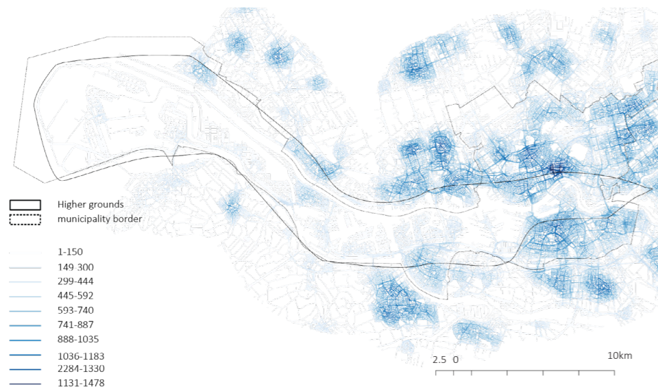
Figure 85 | The centralities of the network based on the amount of streets within reach. (Image by author, using PST tool)
