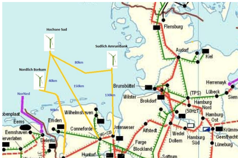
Figure 6. 9: Multi-terminal VSC-HVDC network for interconnection of the German Offshore wind farm zones (type 2)
