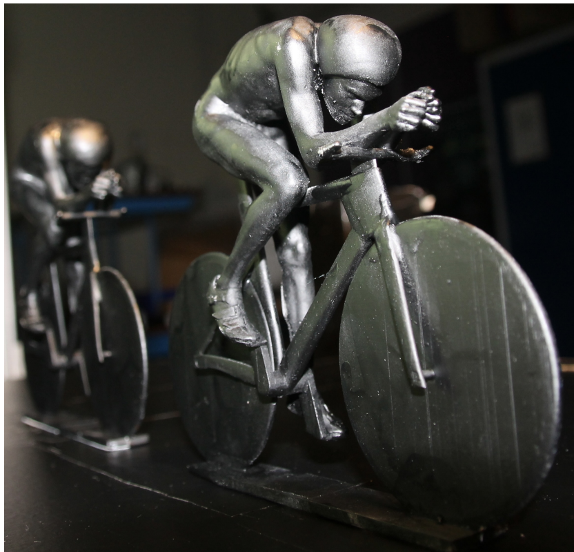
Figure B.1: Surface finish of the 3D printed cyclist model. In this figure, the models have been coated in black mask paint for the PIV campaign
