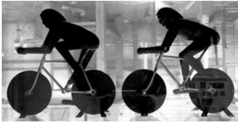
Figure 3.3: 1/10 scaled model used in a water tank for PIV testing (Barry et al. 2016a)
