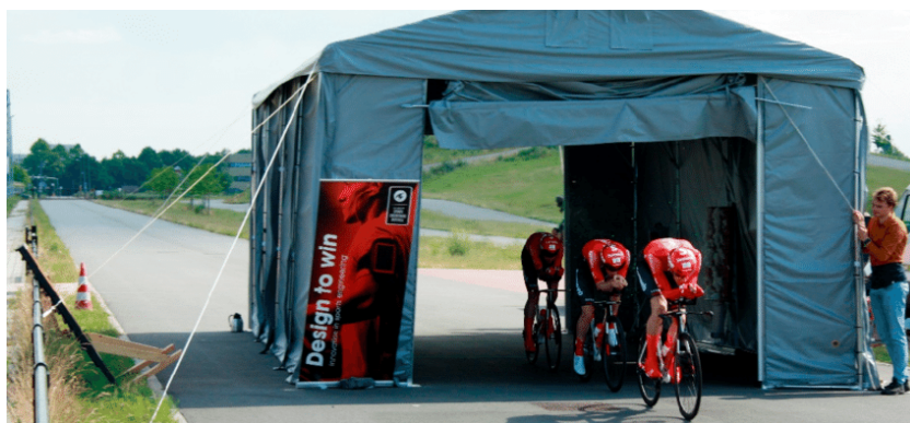
Figure 3.4: Drafting line of cyclists riding through the tent measurement zone for the Ring of Fire experimental method (Spoelstra et al. 2021)
