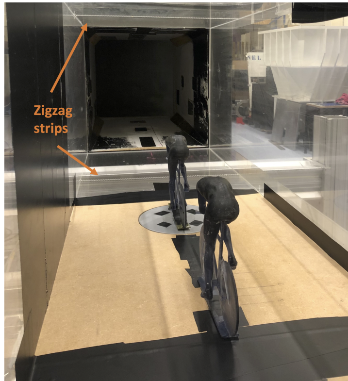
Figure 5.3: Test section configuration for the force balance experiments, with the upstream object being measured. Additionally observable are zigzag strips placed both on the floor and ceiling boundaries upstream of the test area.
