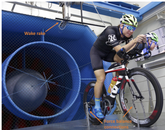
Figure 3.1: Dynamic wind tunnel testing of a pedalling cyclist, using a force balance for drag measurement and pressure probe rake for wake characterisation
