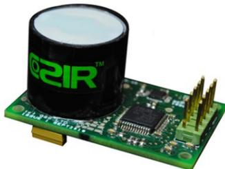
**Figure 2.5:** The CozIR wide range  $\text{CO}_2$  sensor has a range from 0 to 1 000 000 ppm and is used to determine the  $\text{CO}_2$  concentration inside the bell jar. The used sensor has an adapter fitted on top to allow for in-line measurements.
