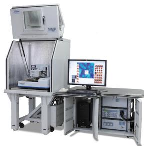
**Figure 2.2:** The Bruker Dimension FastScan is a semi-automatic commercial AFM [16].
