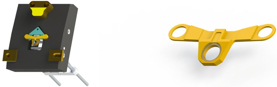
(a) Original cantilever holder for liquid measurements inside the AFM scan head. (b) The original cantilever holder for measurements in liquid.
