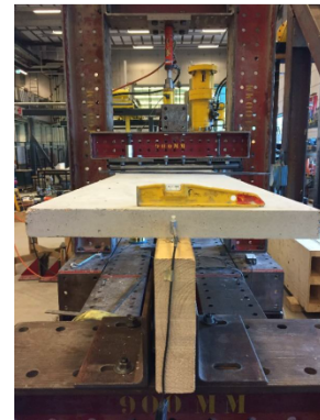
Figure 31: TCC floor during lab test [8]
