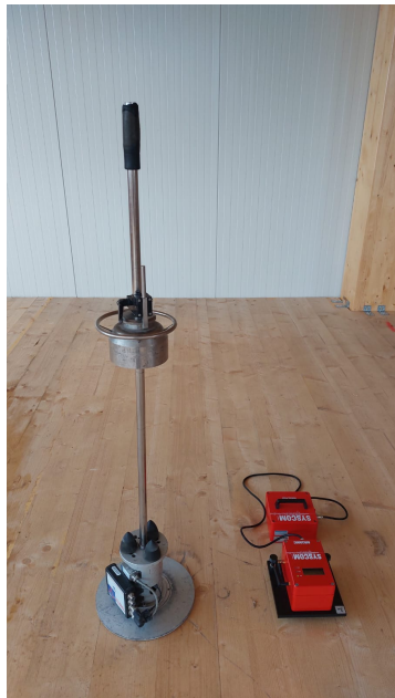
Figure 39: Test setup: Loading mechanism and velocity sensor
