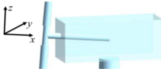
Figure 5.3: Coordinate System of Upwind Wind Turbine in OpenFAST [80]
