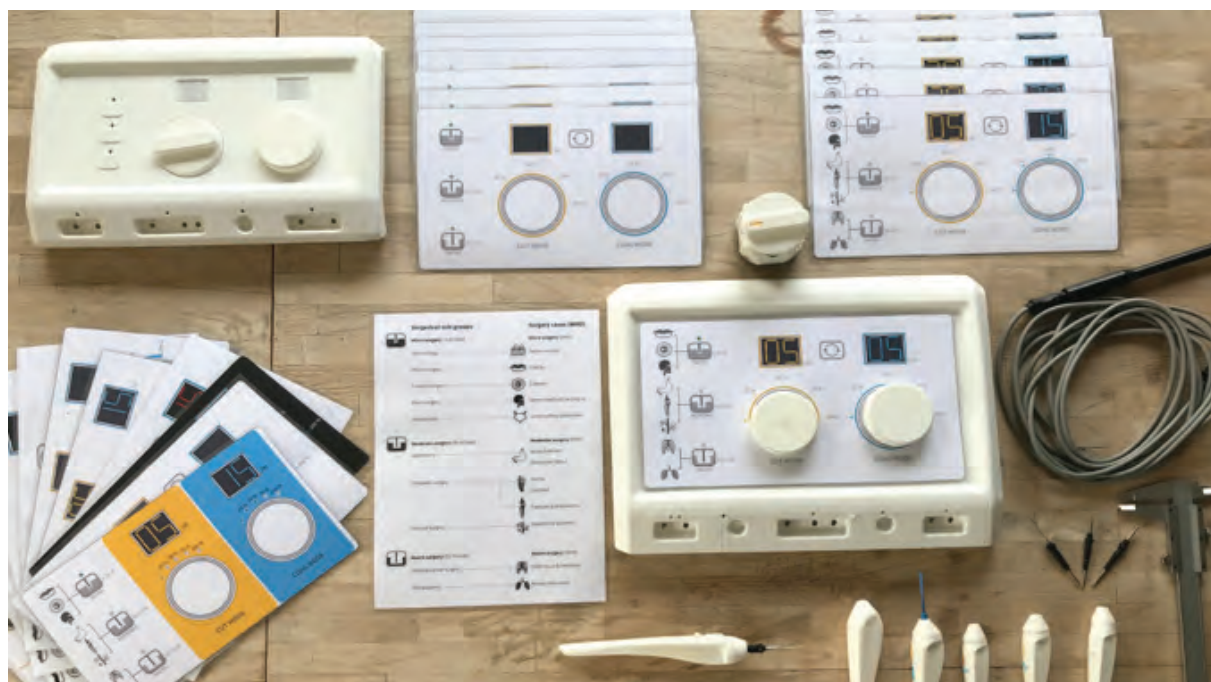
Figure 6.1: Demonstrator designs of the ESU interface and the monopolar handheld that were evaluated by 19 surgeons and 2 BMETs working in Kenya (Study 4, Table 6.1).
