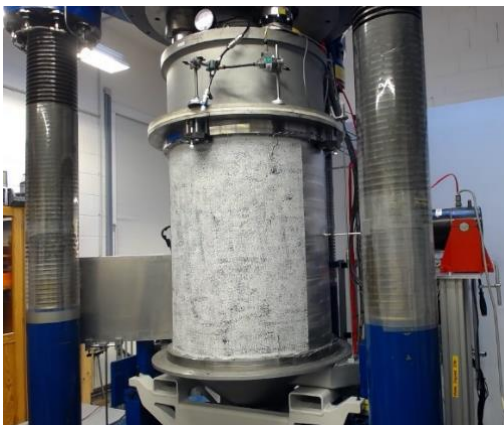
Figure 5 - Left: Metallic structure in the DLR buckling facility load by axial compression and internal pressure
