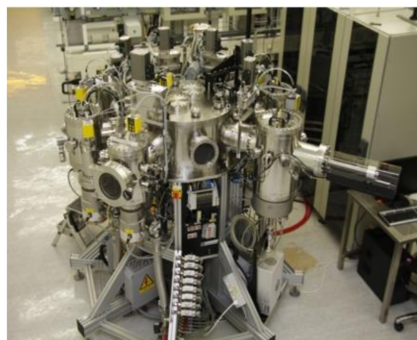
Figure 20: The PECVD equipment used, supplied by Elettrorava S.p.A.
