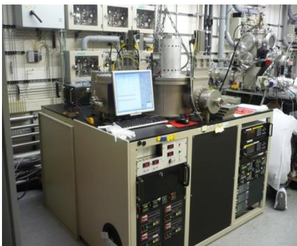
Figure 20: The PECVD equipment used, supplied by Elettrorava S.p.A.
