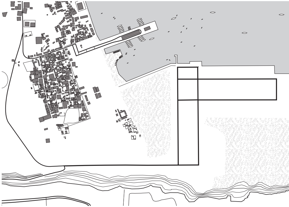
Figure 46: (c. 2005 ) A jetty has been constructed for the fishermen to more easily dock their boats and offload caught fish. The fish market is also located on this jetty as well. The southern end of the East Bay has been filled in as the first phase of port construction. The fish habitats directly in that area are thus gone. The southernmost fisherman's village is now no longer on the beach but is blocked in by the filled in port. New roads have been built that access the port around Mohalla Band.
