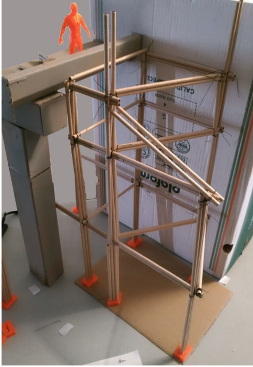
Figure 31: Rudimentary test model to explore the interaction between the flyover and bamboo structure underneath; supported by an overturned orange crate.
