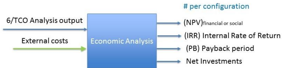
Figure 5-14: Economic analysis sub-block operation principle
