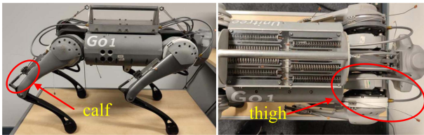
Fig. 9. Two views of the E-Go robot, a Unitree Go1 robot enhanced with springs acting in parallel to all the 12 joints. The springs acting in the sagittal plane for the E-Go robot are highlighted.
