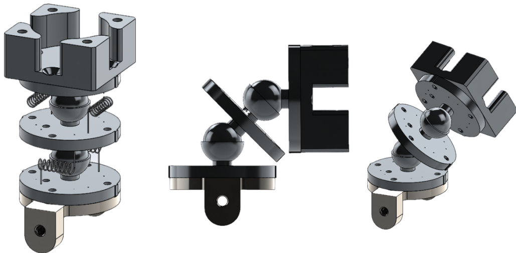
Figure 1: SolidWorks model of a concept surrogate neck design using a ball and socket joint in combination with torsion springs, including Q0 mounts
