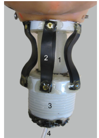
Figure 3: Surrogate neck by Sullivan et al. [17]; 1: Silicone body, 2: Double neoprene rubber bands, 3: Threaded connector, 4: Tygon tubing
