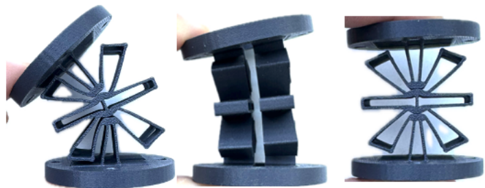
Figure 18: From left to right; flexion/extension, lateral bending, compression of prototype PETG-CF5
