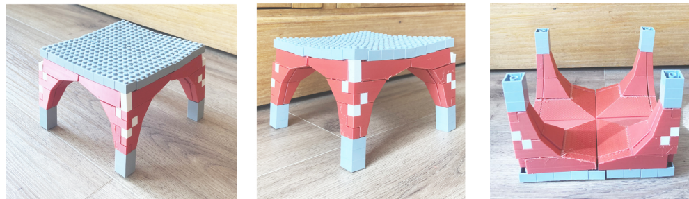
Figure 28: Second iteration for prototyping with 3d printed blocks: full vault
