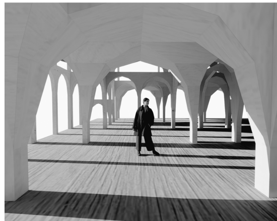
Figure 1: Vault prototype and render images, by Author
