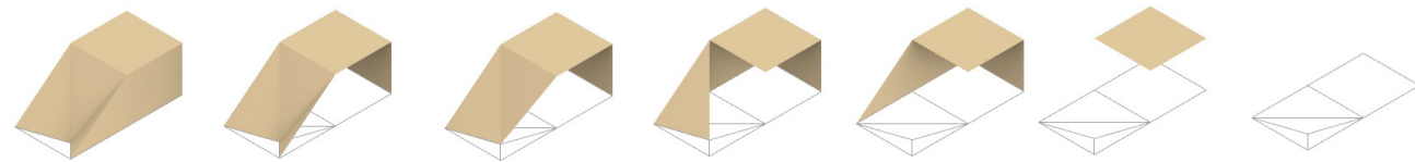
Figure 41: Approximation of a geometry, shaping the voxels with mesh cuts, Author
