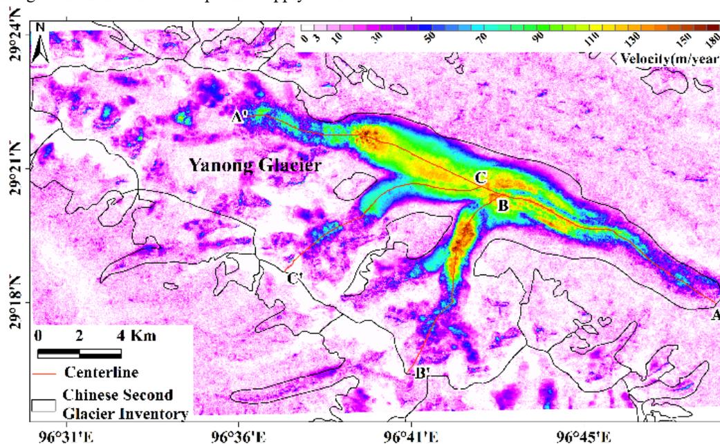
Figure 3. Stack velocity of the annual velocity field in Yanong Glacier from 2013-2018.
