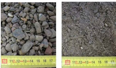
Figure 2. Products from crushed concrete by ADR: Coarse (left) and Fine (right) [9].
