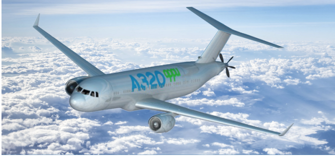
Figure 1.4: Rendering of the conceptual design of the next generation A320 aircraft with integration of the APPU system, showing the modified empennage and aft-mounted auxiliary propulsor in boundary layer ingestion configuration.
