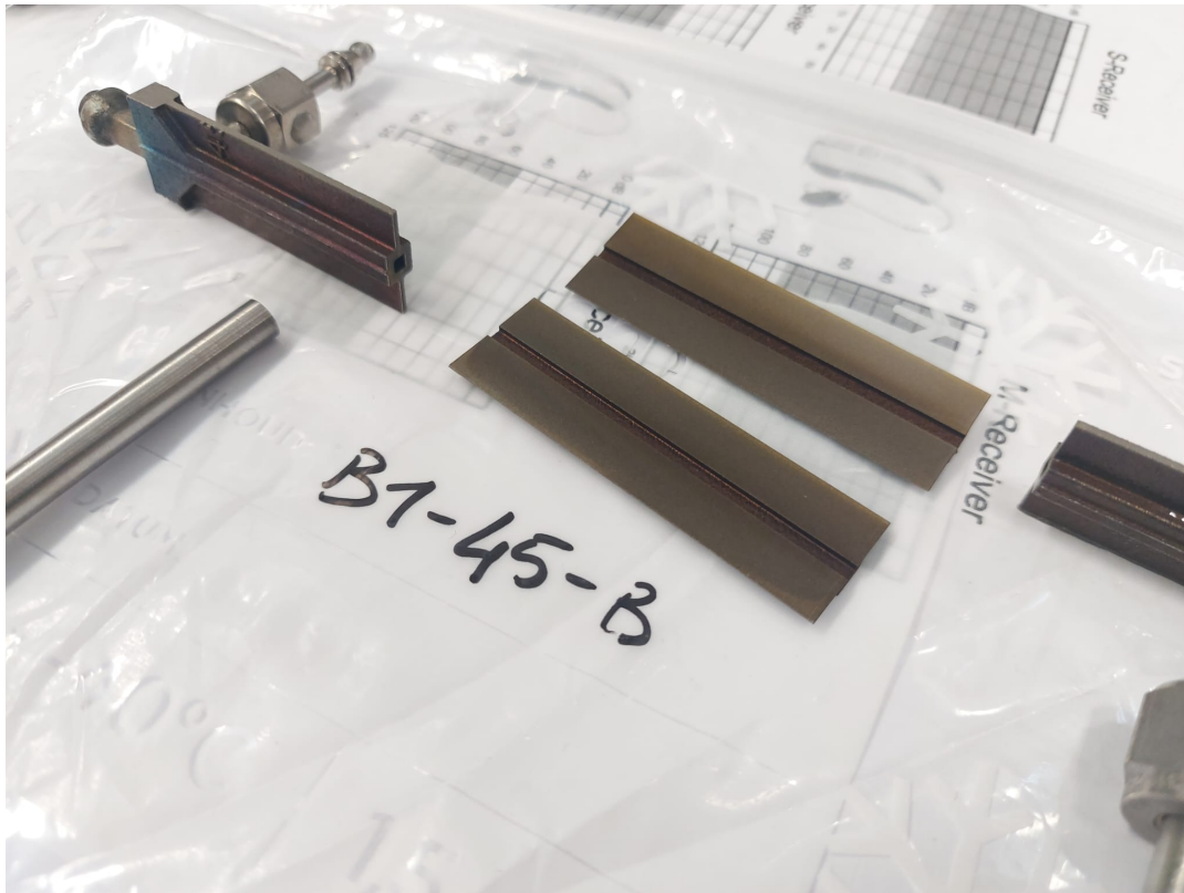
Figure 3.13: Channel B1-45-B, processed for microscope analysis
