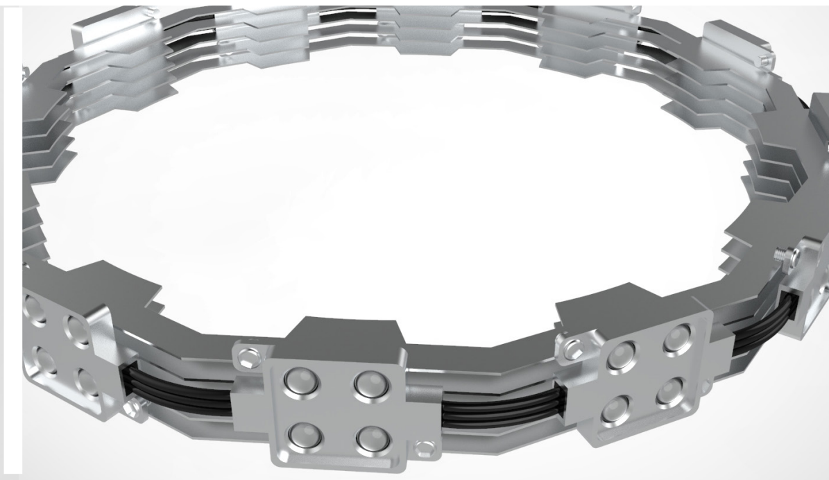
Figure 16.8: The ring with LED modules, linked in serie
