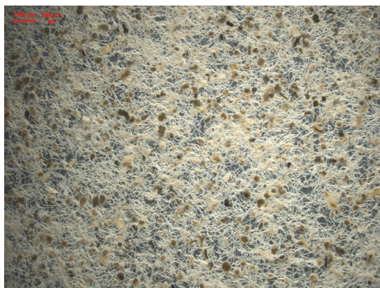
Figure 11.16 Image of sieved ( \geq 200\mu\text{m} ) excess sludge from a full-scale Nereda ® plant showing cellulose fibres meshed with pieces of granular sludge.
