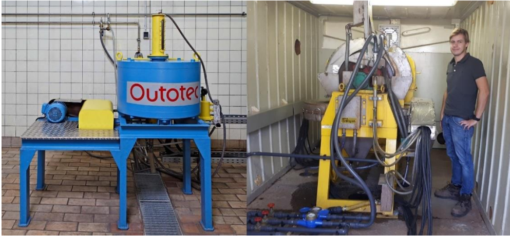
Figure S4.2: Left : Slon-100 bench-scale VPHGMS. Picture courtesy of Outotec. Right: Slon-750 pilot-scale VPHGMS. Wokke (172cm) for scale.
