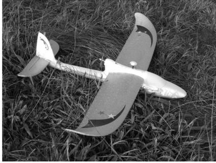
(a) The Easystar model airplane that is used as the flying test platform for the mini UAV system.
