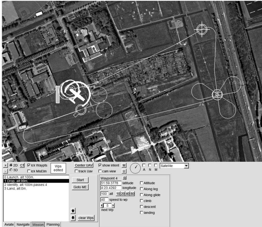
Figure 5.9: A mission is shown on the map of the UAV GCS. It consists of the following mission elements: launch, paintball drop, identify, and land. The UAV is in a circular holding pattern above the launch area. The predicted flight path is shown for the mission.
