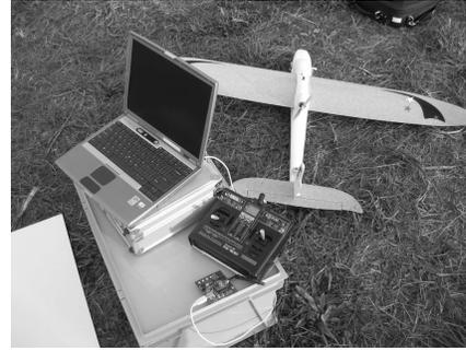
(b) The Easystar, a laptop computer as the GCS, the long range modem, and the safety pilot's radio transmitter.
