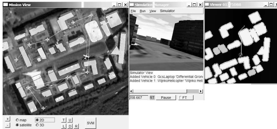
Figure 5.14: The SmartUAV interface at the aviate level. The left window shows the map with the flight plan in terms of waypoints, the flown path, the computed path, and the obstacles as high cost areas on the map. The middle window is a simulated view from the UAV. The right window is a visual representation of the actual cost map that the algorithm uses.
