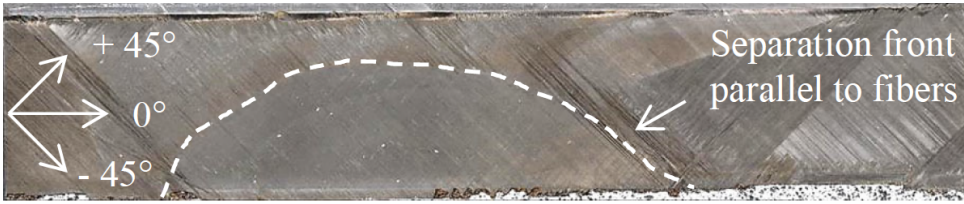
Figure 6.16: Post-mortem interface seen from skin side of 4PT2.
