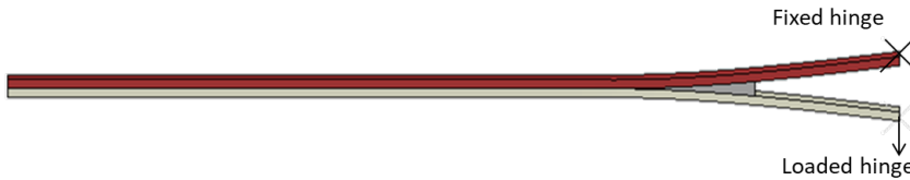
Figure 2.9: Double cantilever beam design
