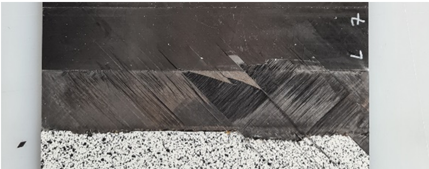
Figure 5.19: Top view of the interface from skin side post-mortem, showing that the top ply is partially peeled off.
