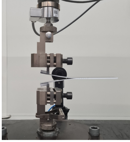
Figure 3.4: Setup for double cantilever beam. The load is applied on the left with the bottom clamp moving downwards.
