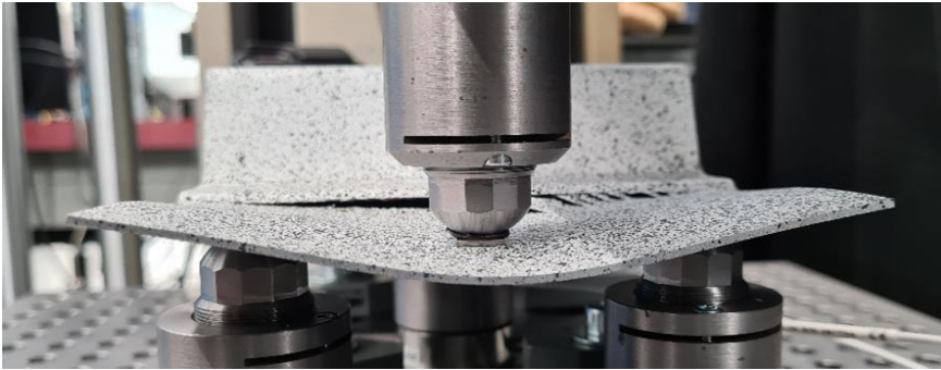
Figure 5.18: Side view of physical separation showing migration from the interface into the top skin ply.
