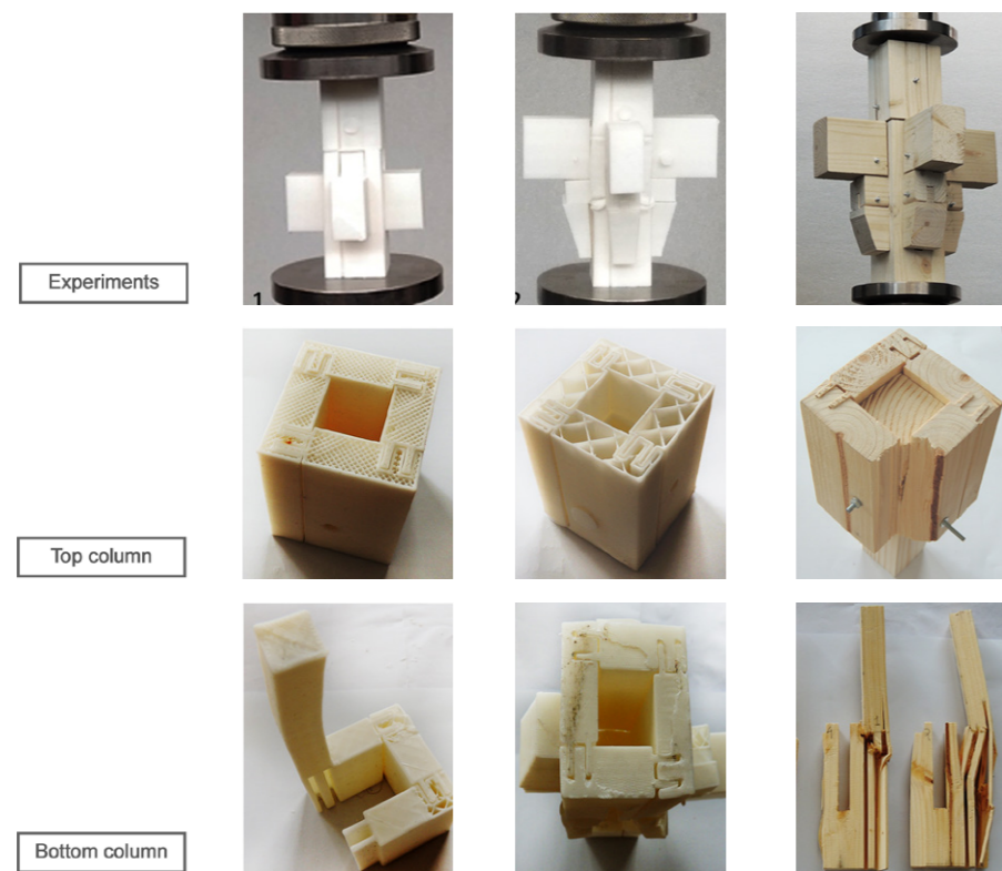
Figure 8.17: Effect of compression test on the box column joinery during the experiments.
