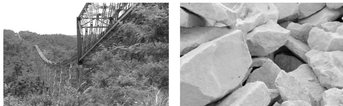
Figure 4.9: Left – 17 km conveyor belt built by Lafarge group for transporting limestone across Indo-Bangladesh border. Right - extracted limestone in a quarry. (Source: http://i.imgur.com/cWYPvYU.jpg and thefinancialexpress.com )
