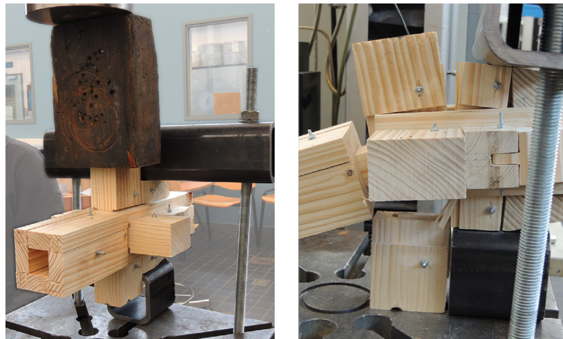
Figure 8.47: Before and after images of 3 simultaneous lateral cyclic loading test for specimen 4 – softwood
