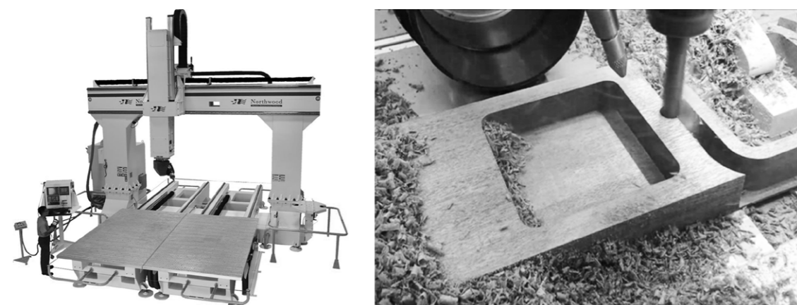
Figure 6.15: Left – 5 axis CNC milling machine (northwoodmachine.com). Right – CNC milling on wood in progress (https://www.youtube.com/watch?v=xtDLmrrmX3Q).
