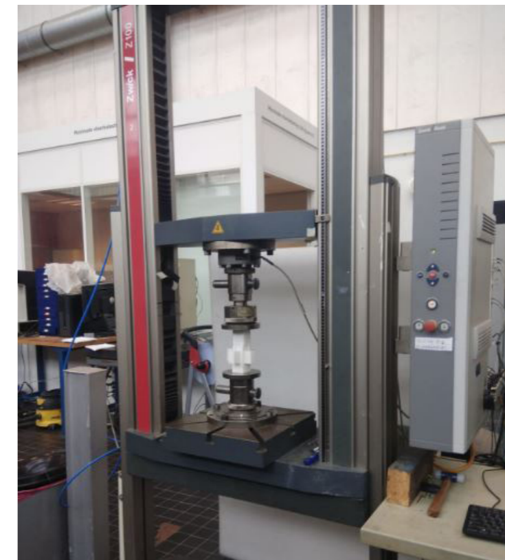
Figure C.2: Showing the test setup for vertical loading using Zwick/ Z100
