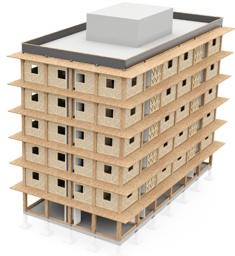
Figure 10.3w: Proposed timber construction system.
