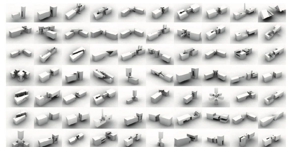
Figure 6.13: Typical types of traditional Japanese joineries (Kanasaki & Tanaka, 2013).
