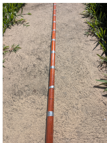
(b) Measuring stick marked at 10 cm intervals (own image)
