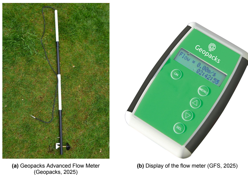
Figure C.2: Geopacks Advanced Flow Meter and its display
