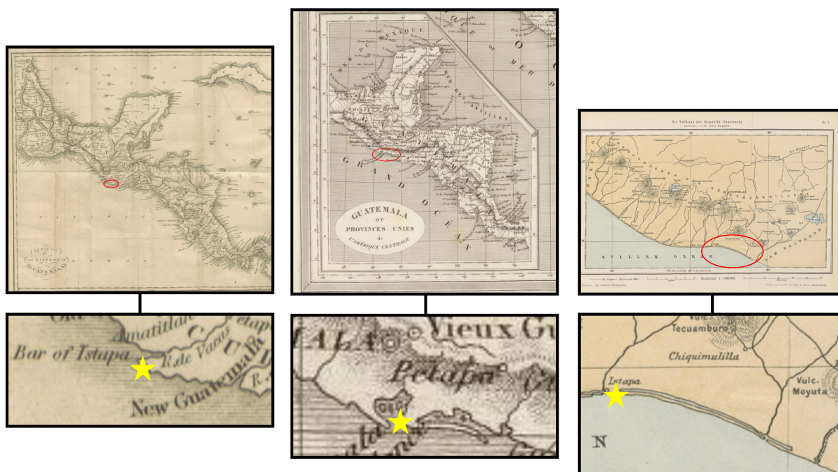
Figure 3.15: Maps of developing spit at the same location. The maps are from the years 1823, 1837 and 1895, respectively. Lower maps are zoomed in. The yellow star represents a reference point at the mouth of river Maria Linda close to the town of Iztapa (Aubree, 1837; SAPPER, 1895; unknown, 1823).
