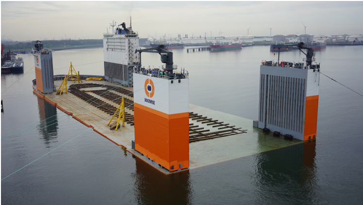
Figure 6.1: Guidepost (yellow tripods) and cribbing beams on HTV deck
