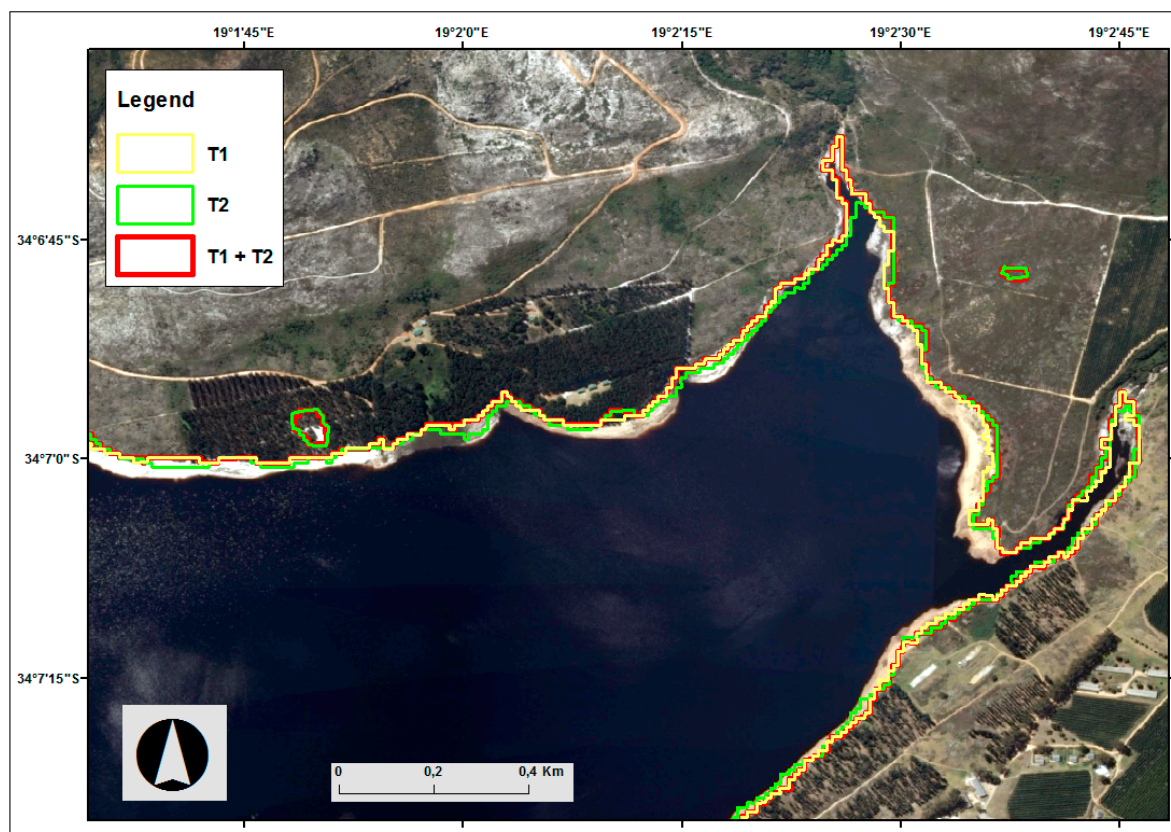
Figure 6. Visualisation of water masks derived from T1 (NDWI), T2 (SAR VH polarisation), and T1+T2 (fusion of T1 and T2). The background image is an aerial photograph taken in November 2014 when water levels were very low.
