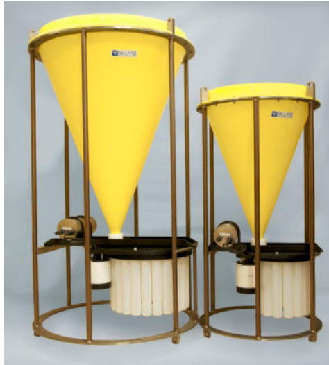
Figure 2.7: Common sediment trap design [48]
