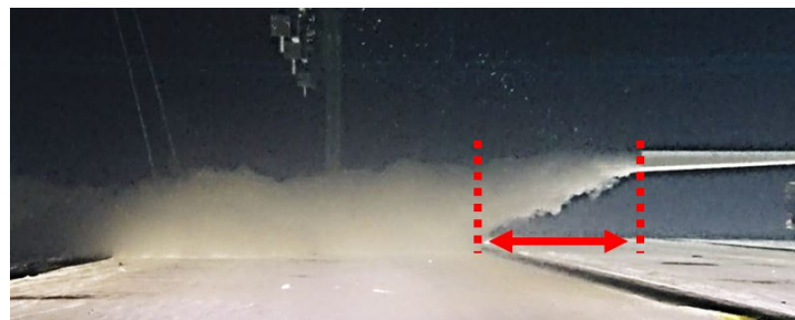
Figure 4.6: Definition of the impingement length
