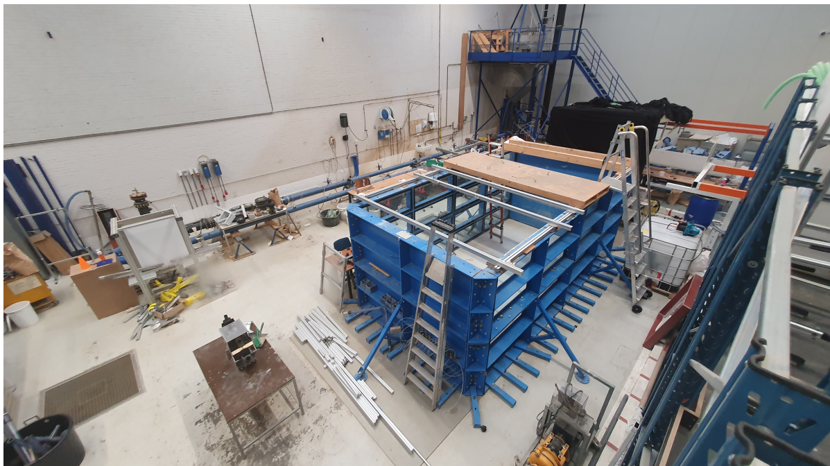
Figure 3.1: Dredging lab with modular flume
