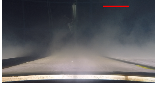
Figure 5.5: Suspended sediment experiment 3, 6 sec after discharge. Including marker for max height
