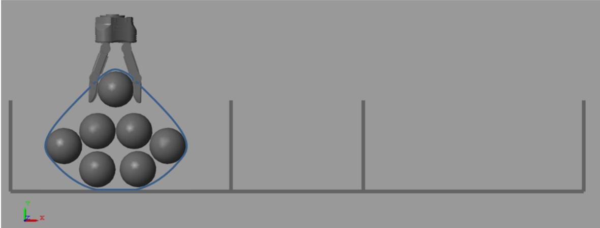
**Figure 6-19:** The simplified version of the virtual net with oranges and the gripper in 2D in the pick-and-place environment. The virtual net is indicated in blue for clarity, but not present in the real simulation.
