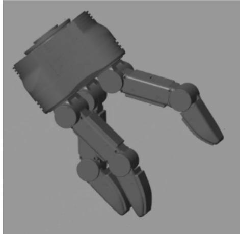
**Figure 5-2:** The 3D model of the Schunk SDH gripper that is used in simulations.
