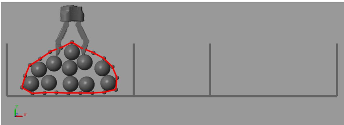
**Figure 5-10:** The virtual net with oranges and the gripper in 2D in the pick-and-place environment. The connections between the particles of the net are indicated in red for clarity, but not present in the real simulation.
