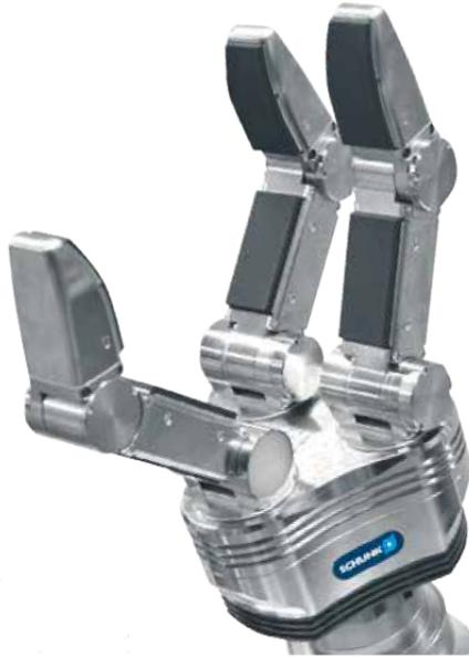
**Figure 2-4:** The Schunk Dextrous Hand (SDH), from [3].
