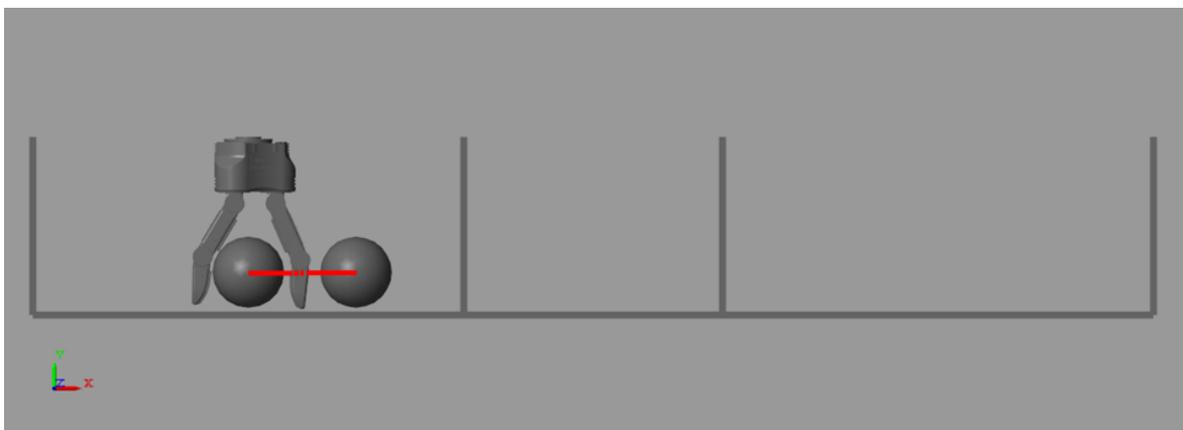
**Figure 5-9:** The virtual pendulum and the gripper in 2D in the pick-and-place environment. The connection between the balls is indicated in red for clarity, but not present in the real simulation.
