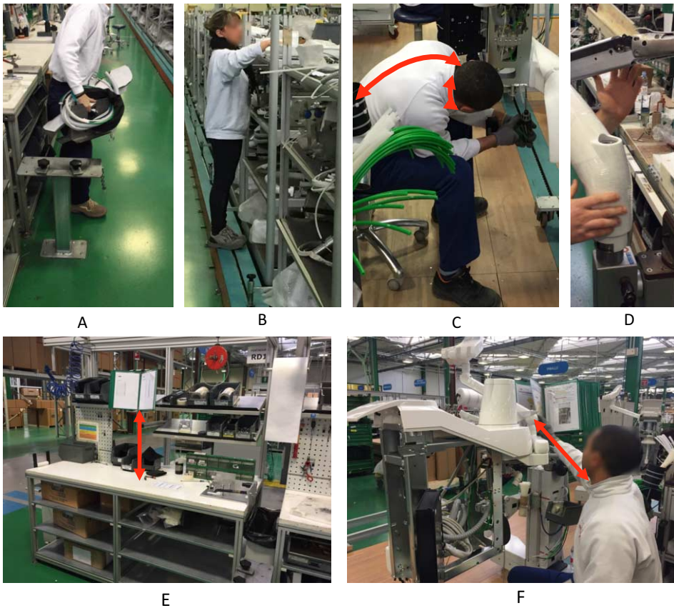
Figure 3. Examples of the human-related criticalities during the assembly process in the case study
