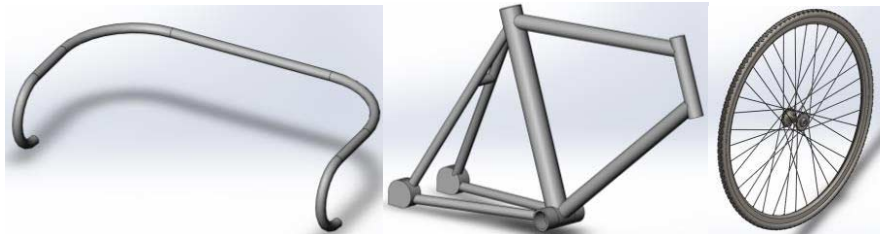
Figure 2. CAD model of handlebar, frame and wheel.
