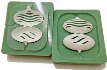
Figure 2. Stratasys 3D printed mould [10].
