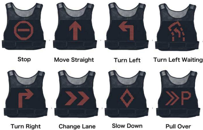
Figure 8. Traffic instructions using images displayed on the vest.
