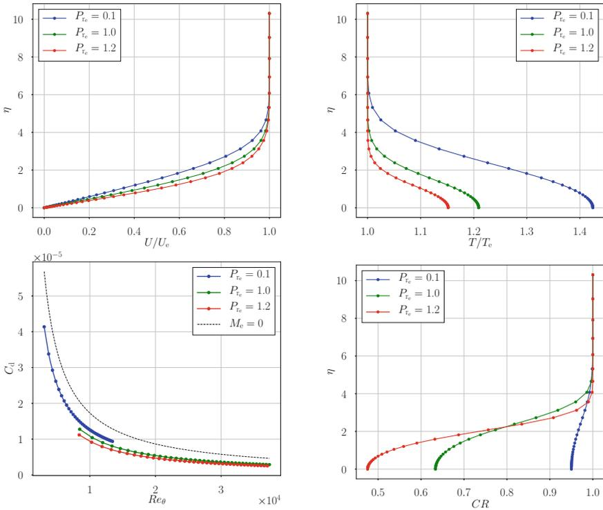
**Fig. 4.** Results for CO<sub>2</sub> in ideal and NICFD conditions at  $Me = 2$ . Top: dimensionless velocity and temperature distribution. Bottom: dissipation coefficient and Chapman-Rubensin parameter within the boundary layer.
