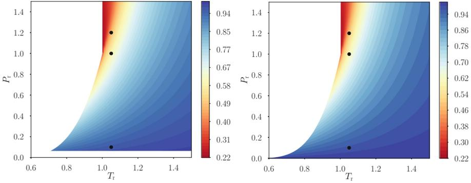
**Fig. 1.** Contours of compressibility factor  $z$  of  $\text{CO}_2$  and Siloxane MM. The black dots indicate the reduced conditions of the flow at the edge of the boundary layer considered in the present study.
