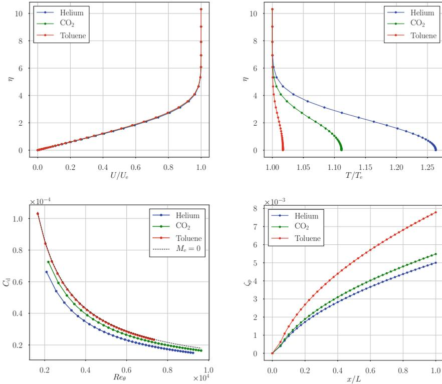
**Fig. 3.** Dimensionless velocity and temperature profile, dissipation coefficient, and global loss coefficient for Helium, CO<sub>2</sub>, and Toluene at  $M_e = 1$ . The dashed line in the  $C_d$  plot refers to the trend for incompressible flows given in [1].
