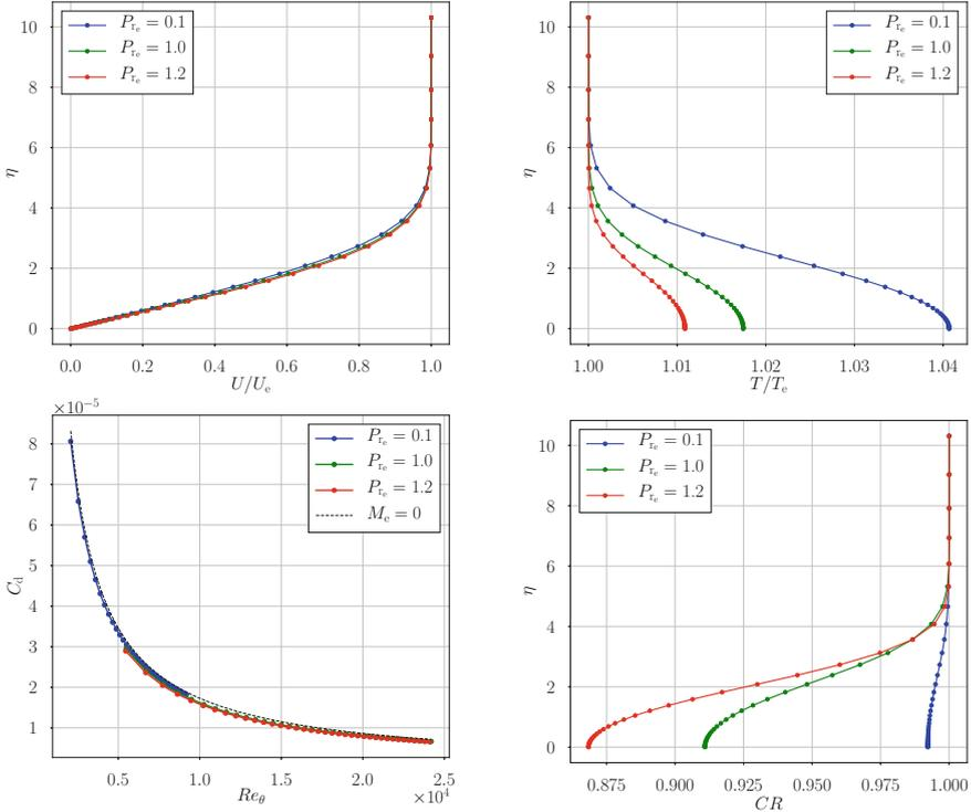
**Fig. 5.** Results for MM in ideal and NICFD conditions at  $M_e = 2$ . Top: dimensionless velocity and temperature distribution. Bottom: dissipation coefficient and Chapman-Rubinsin parameter within the boundary layer.
