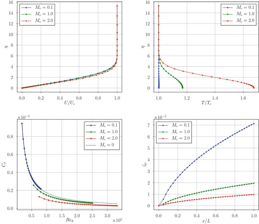
**Fig. 2.** Dimensionless velocity and temperature profile, dissipation coefficient, and loss coefficient for air at three different Mach numbers. The dashed line in the  $C_d$  plot refers to the trend for incompressible flows given in [1].
