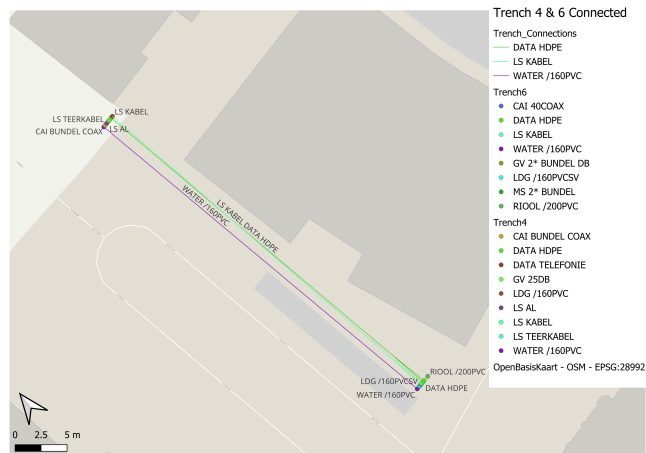
(b) Brammelerdwarsstraat: trenches 4 & 6 final connections
