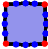
Figure 5: A group of a single pixel with nodes around it. Edge nodes are blue, corner nodes are red.
