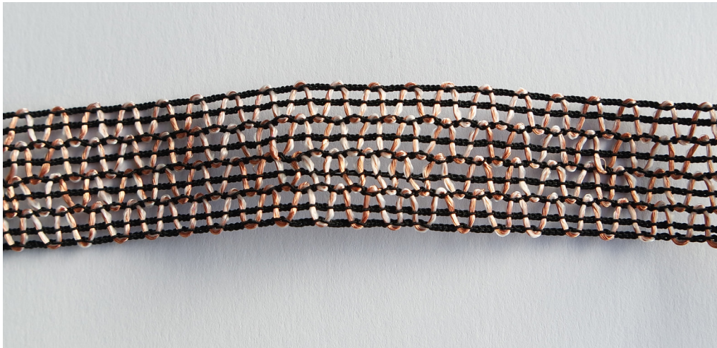
Image 21, Strechy wires (AMOHR tape)
