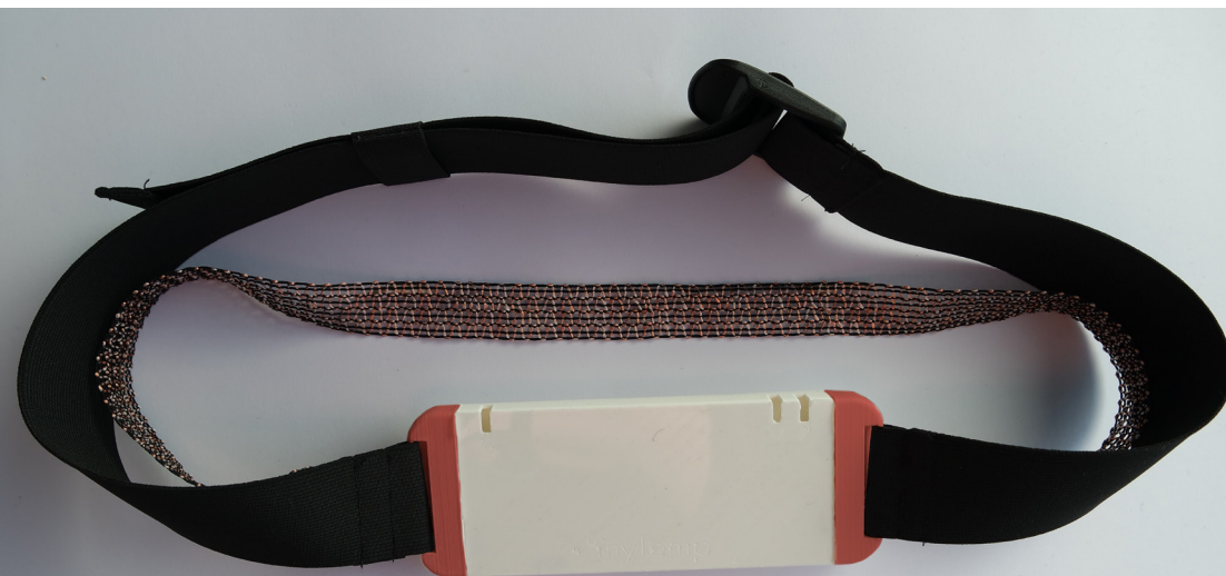
Image 67, Elastic and antenna band connected to the housing
