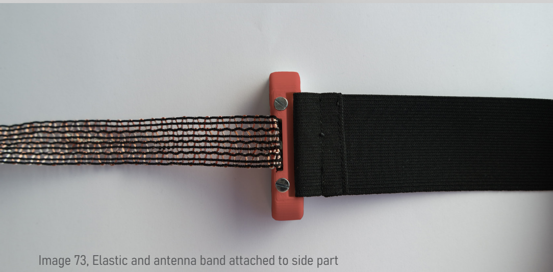
Image 72, Place of attachment of antenna and elastic
