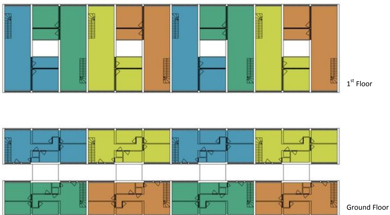
Figure 4.1 – Ground floor and 1st floor of the Tetris Houses. Each color is one apartment.
