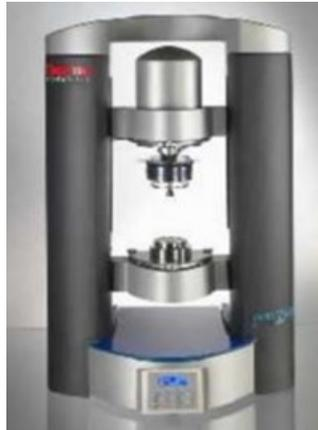
Figure 2.2: Rotational rheometer HAAKE MARS I
