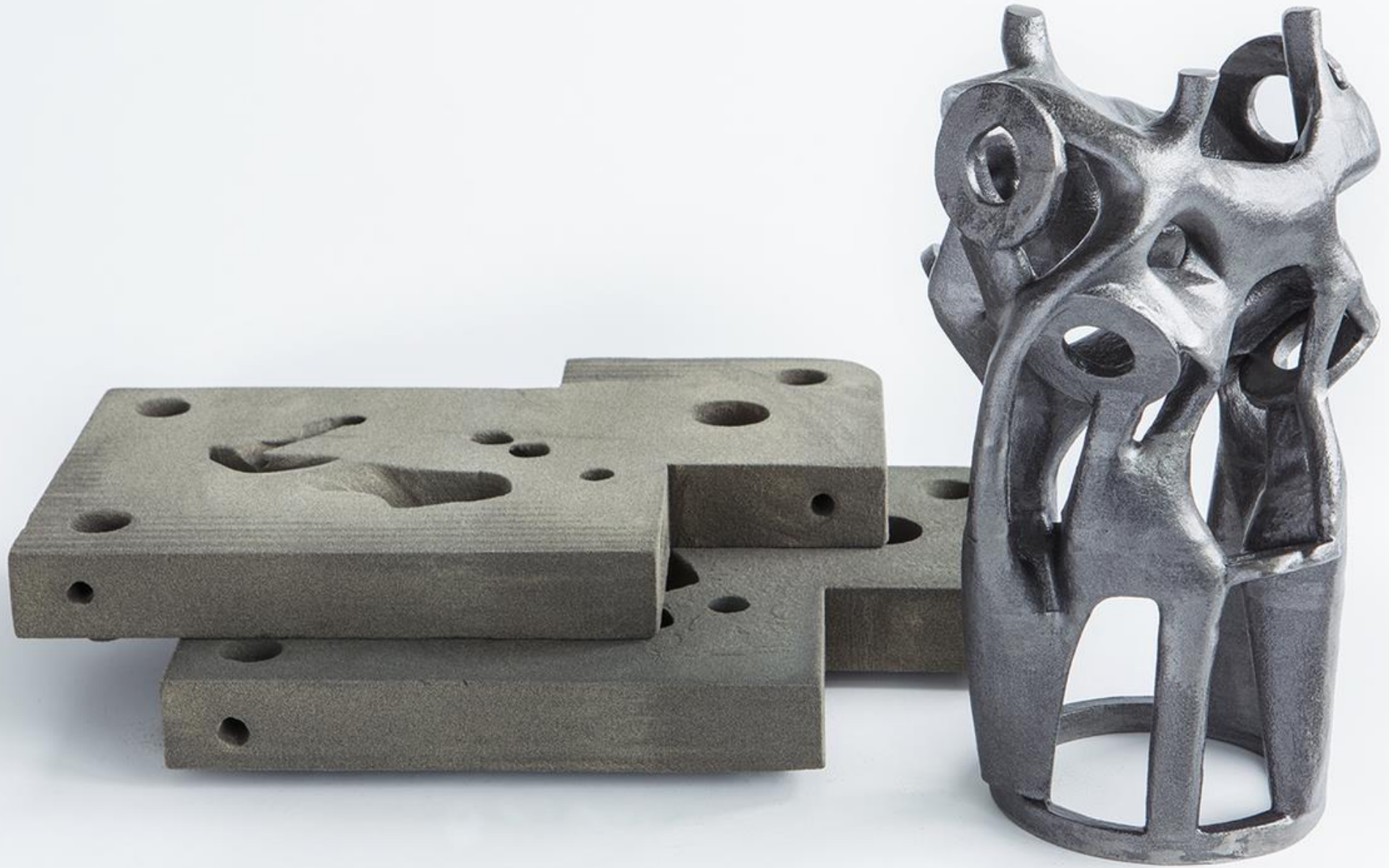
sand mould casting
