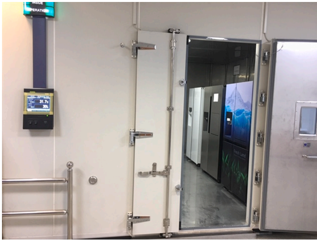
Fig. 5. Walk-in type test room to ensure controlled and constant ambient conditions during experiments.
