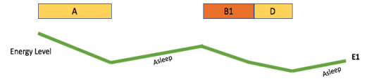
(a) E1 is the energy level of the nominal schedule with no Maximum SOC constraint after all activities up to and including the nominal switch case (A, D, B1) have been scheduled.
