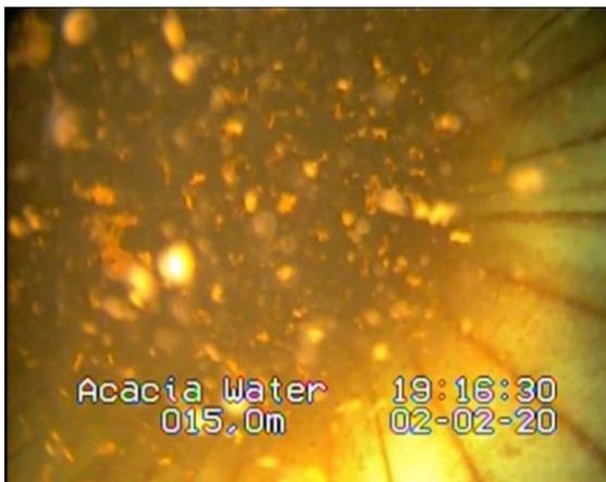
Figure 3.13a: Clogged state after infiltration period one. Image is of the top filter case, taken on February 2<sup>nd</sup>, 2020.
