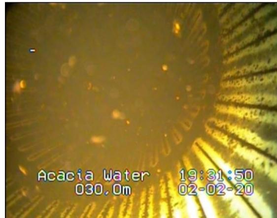
Figure 3.13b: Clogged state of the lower filter case, taken February 2<sup>nd</sup>, 2020.
